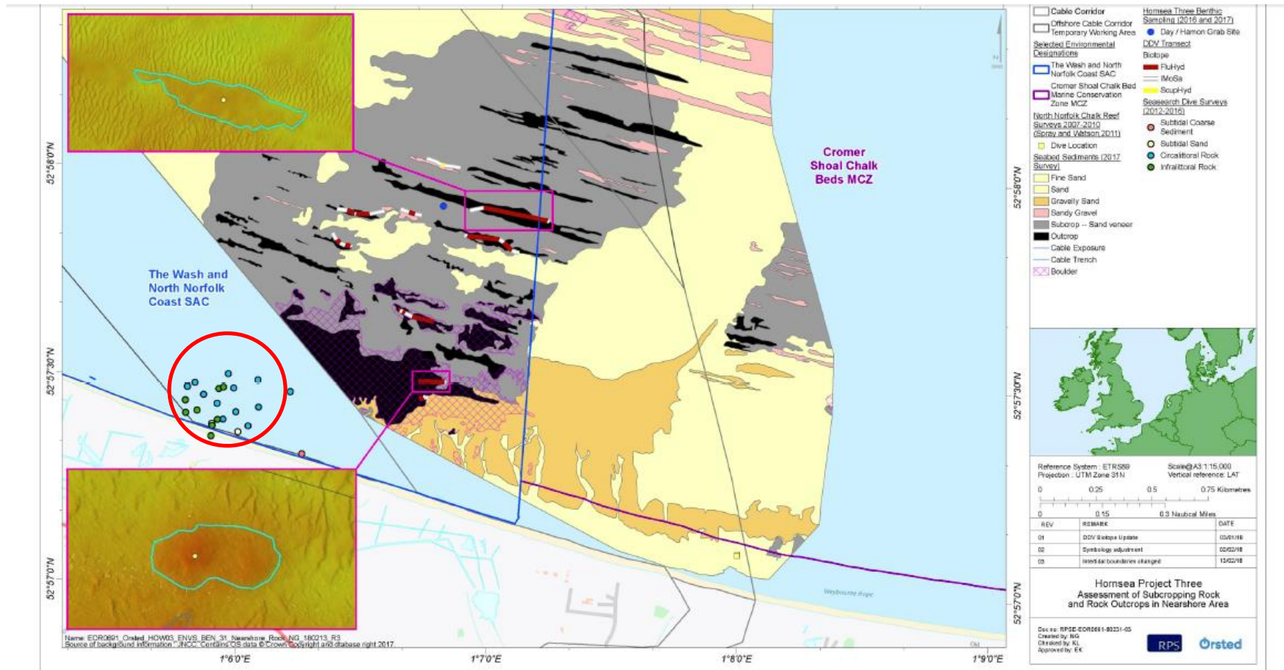
Figure 4.29: Hornsea Three nearshore geophysical seabed interpretation showing subcropping rock (grey) and areas of potential outcrop (black), DDV ground truthing transects with epifaunal biotopes identified and historic records of infralittoral and circalittoral rock in the nearshore area.
