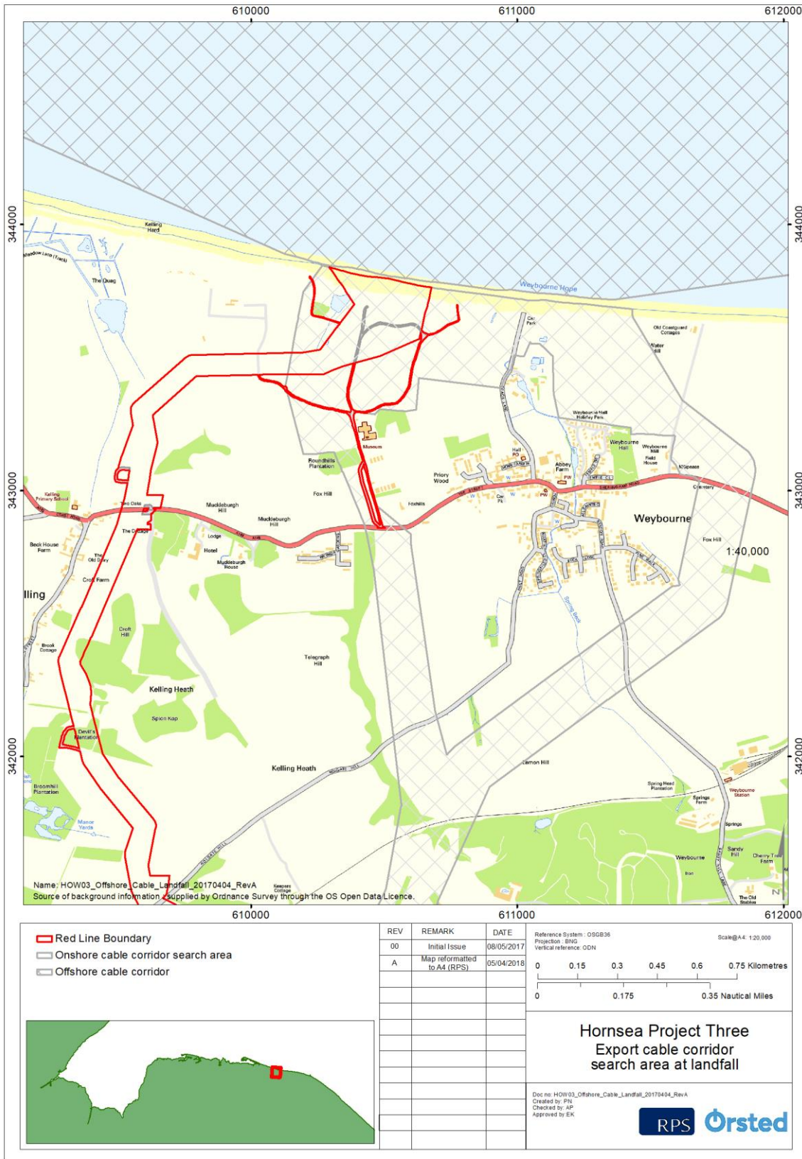
Figure 3.3: Landfall and onshore export cable route corridor.
