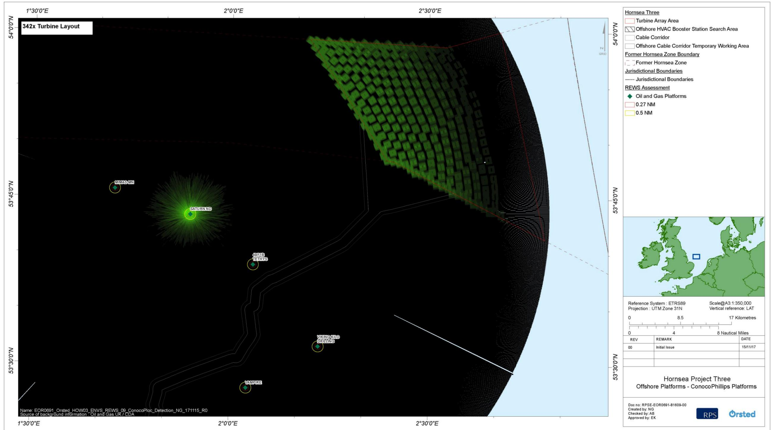
Figure 5.3: Saturn platform REWS detection threshold over the Hornsea Three array area (342 turbines).
