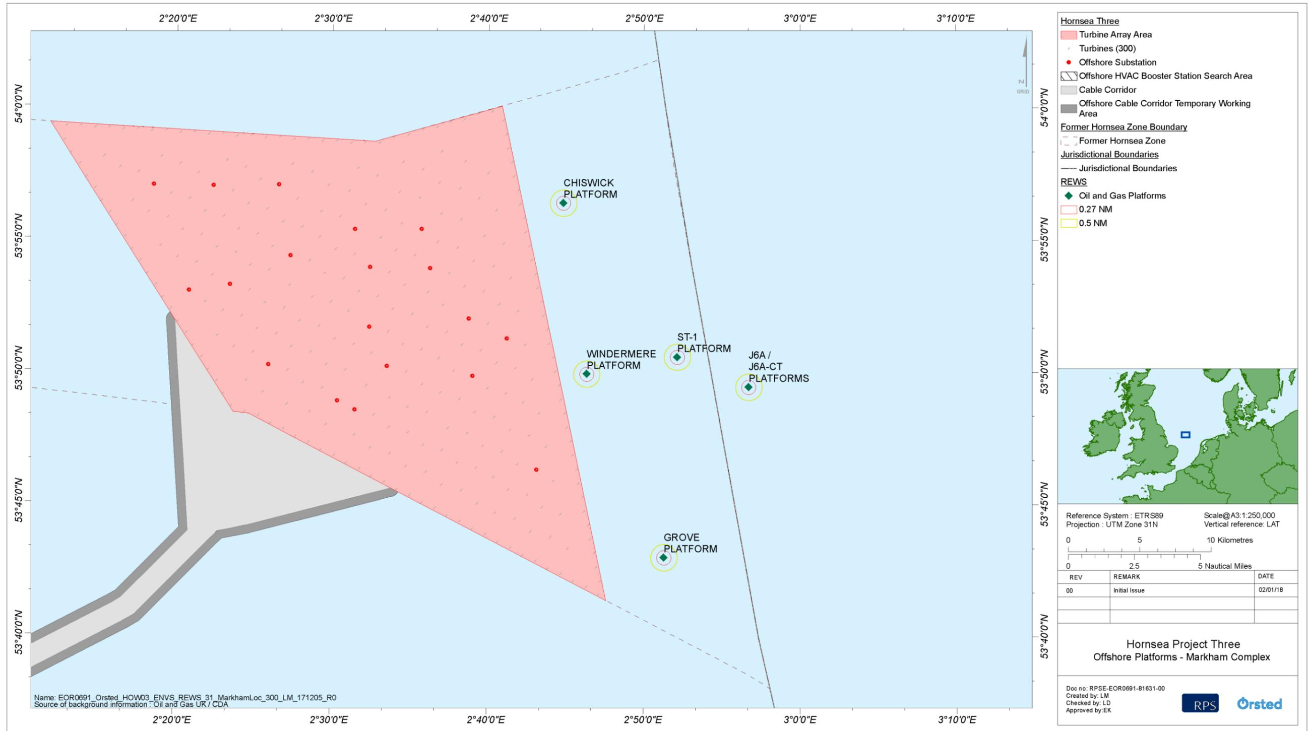
Figure 4.8: Modelled maximum design scenario layout (300 turbines) of Hornsea Three and the Spirit Energy operated Markham complex of platforms.
