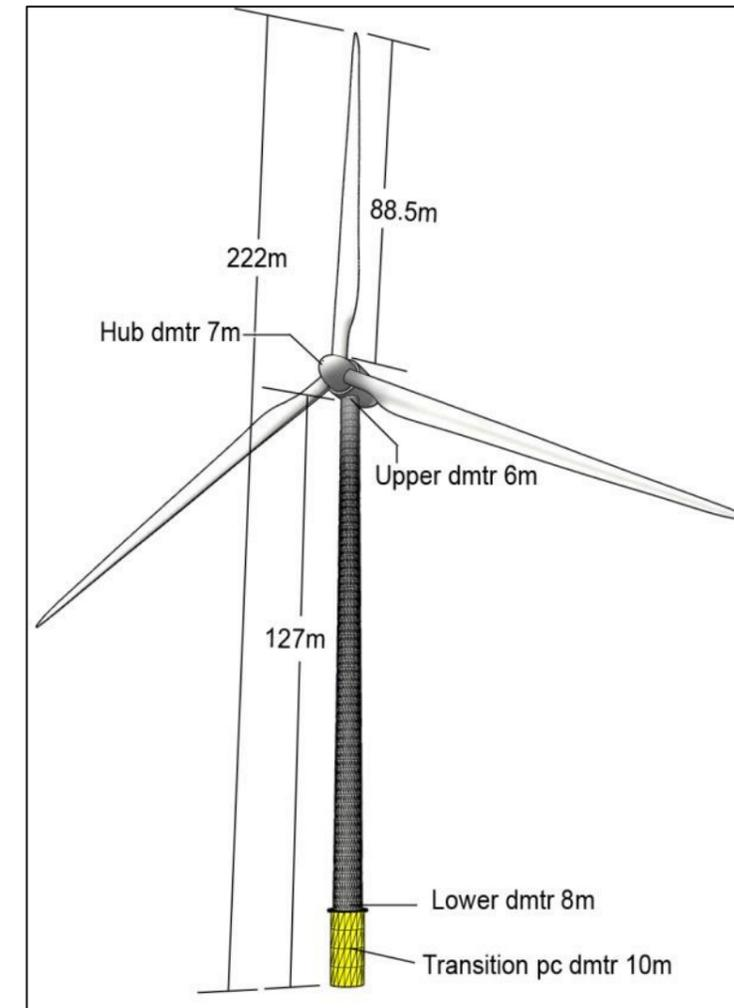
Figure 3.1: Modelled turbine geometry.
