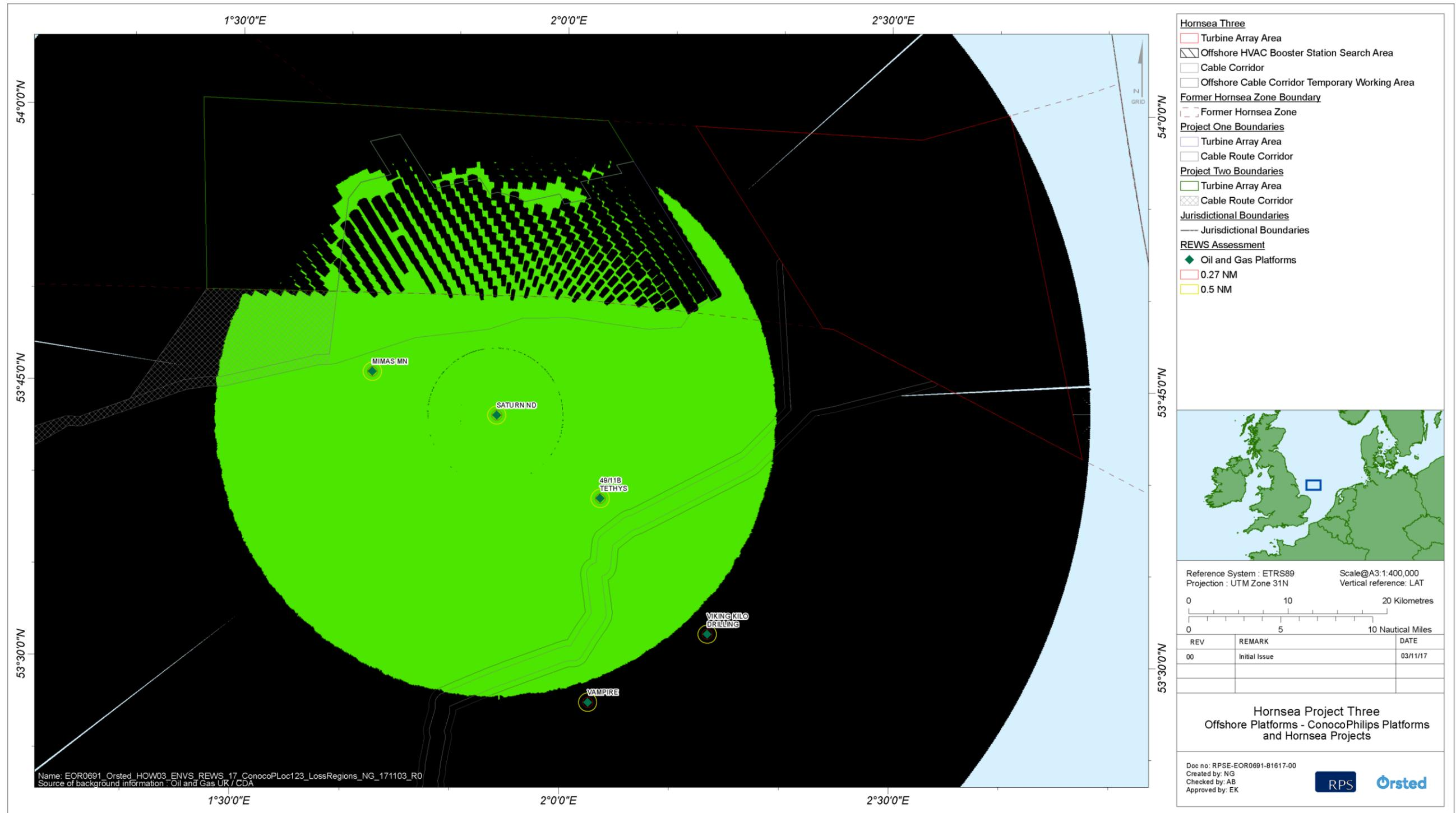
Figure 5.11: Saturn platform REWS detection plot showing loss regions for a 100 m<sup>2</sup> target over the combined Hornsea Project One, Hornsea Project Two and Hornsea Three (342 turbines). (Note that the Hornsea Project One and Hornsea Project Two consented layouts have less turbines than those shown in this figure).
