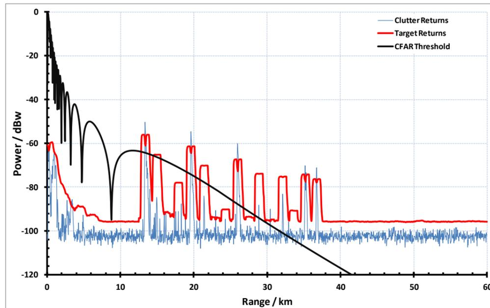
Figure 4.6: Power received from small target at 270° bearing angle.
