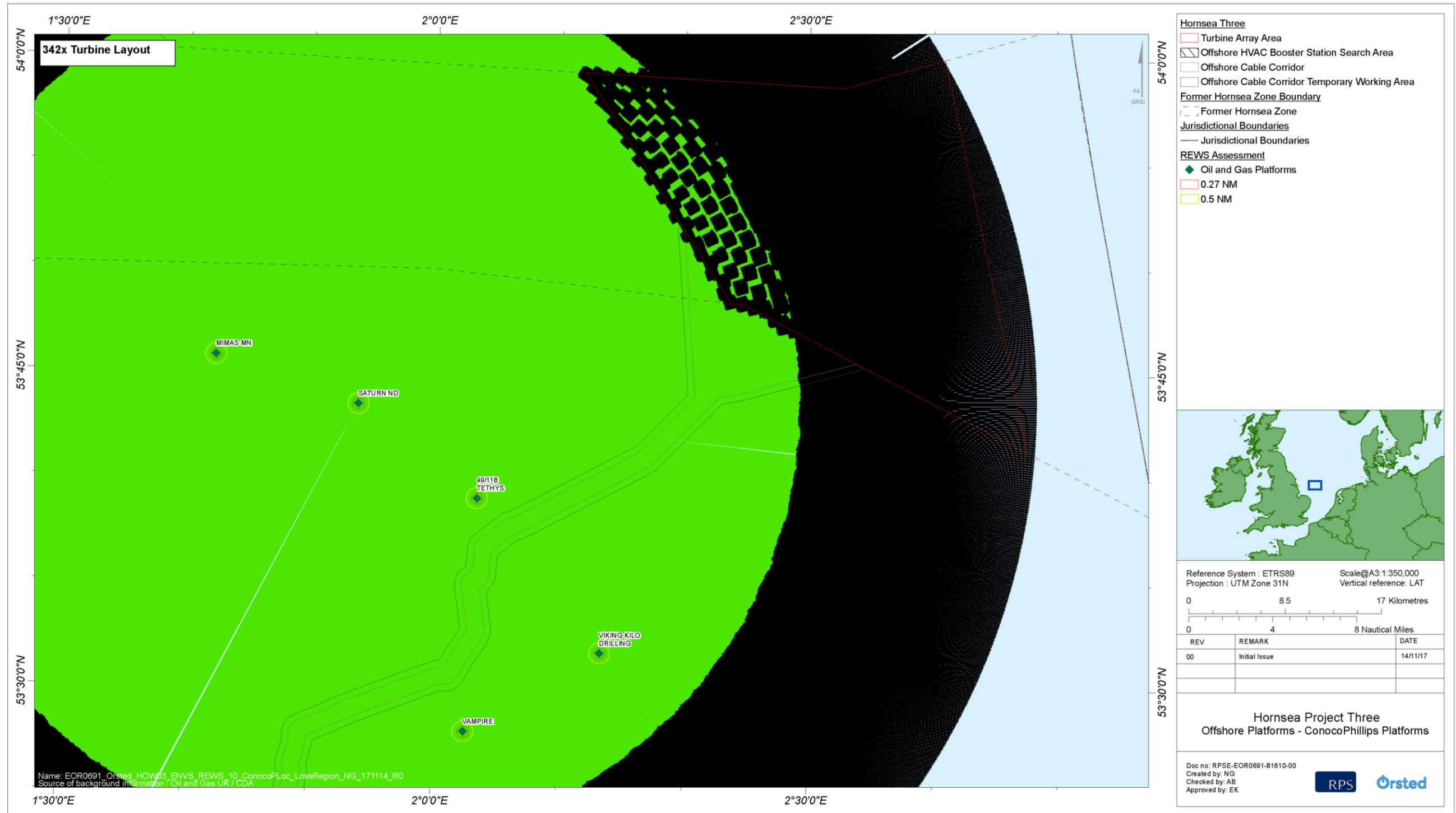
Figure 5.5: Saturn platform REWS detection plot showing loss regions for a large 1000 m<sup>2</sup> RCS target over the Hornsea Three array area (342 turbines).
