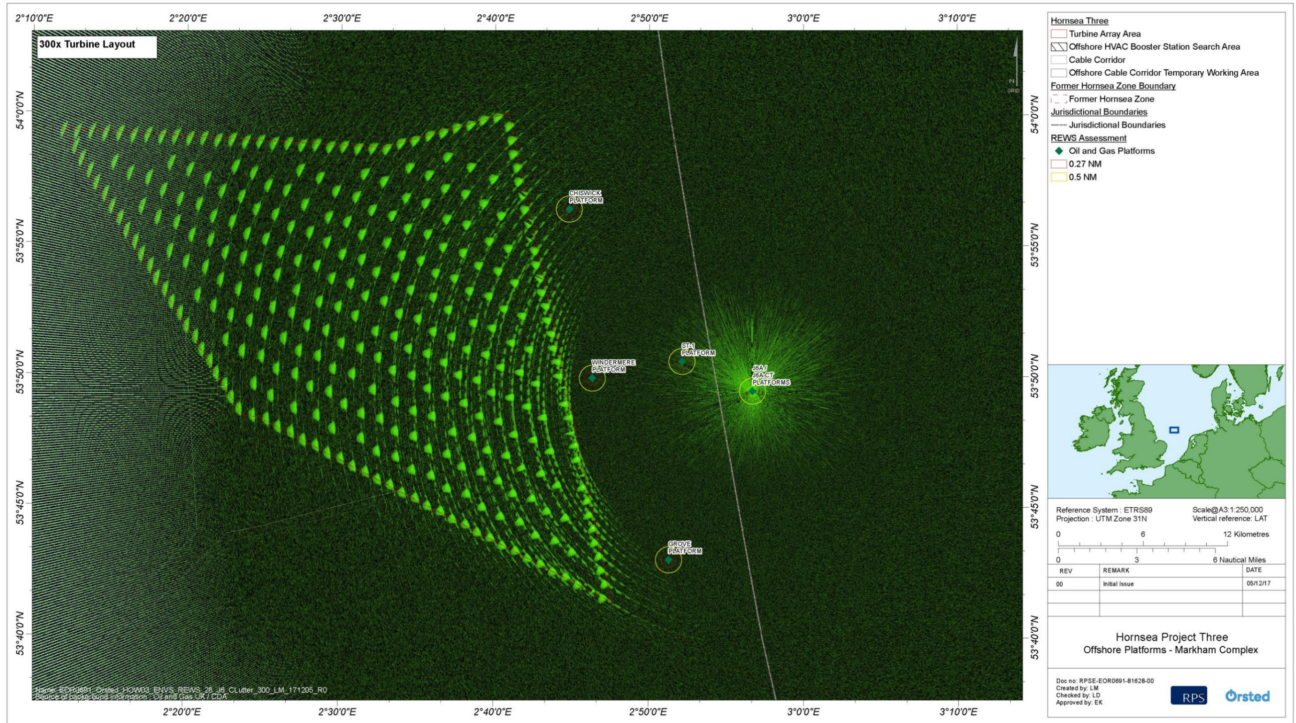
Figure 4.9: J6A platform REWS clutter map showing returns from 300 turbines and sea clutter.
