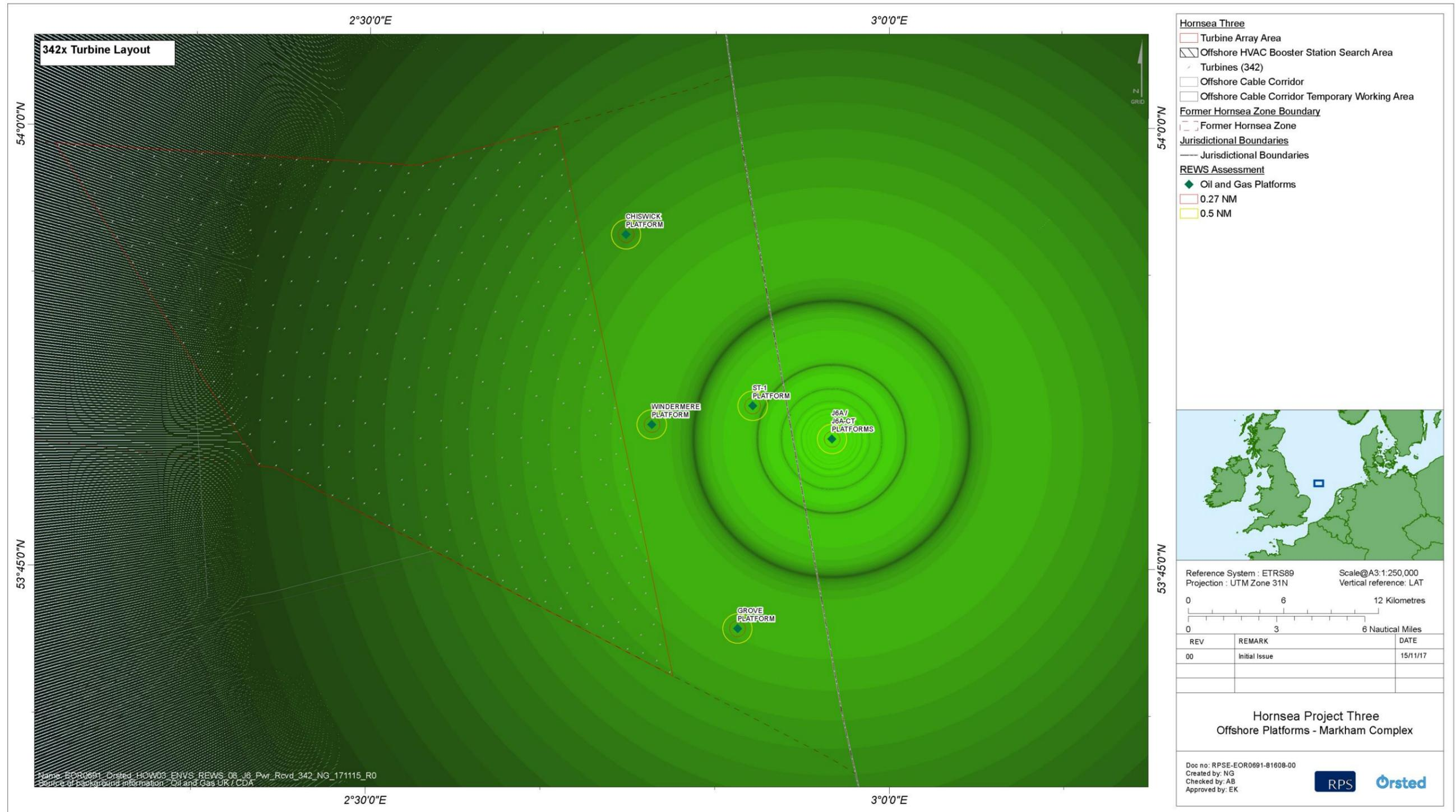
Figure 4.4: Modelled power received from 100 m² target (coverage).
