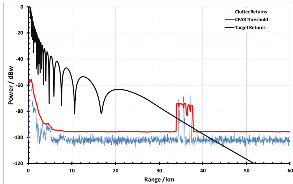
Figure 5.6: Power received from large target at 39° bearing angle.
