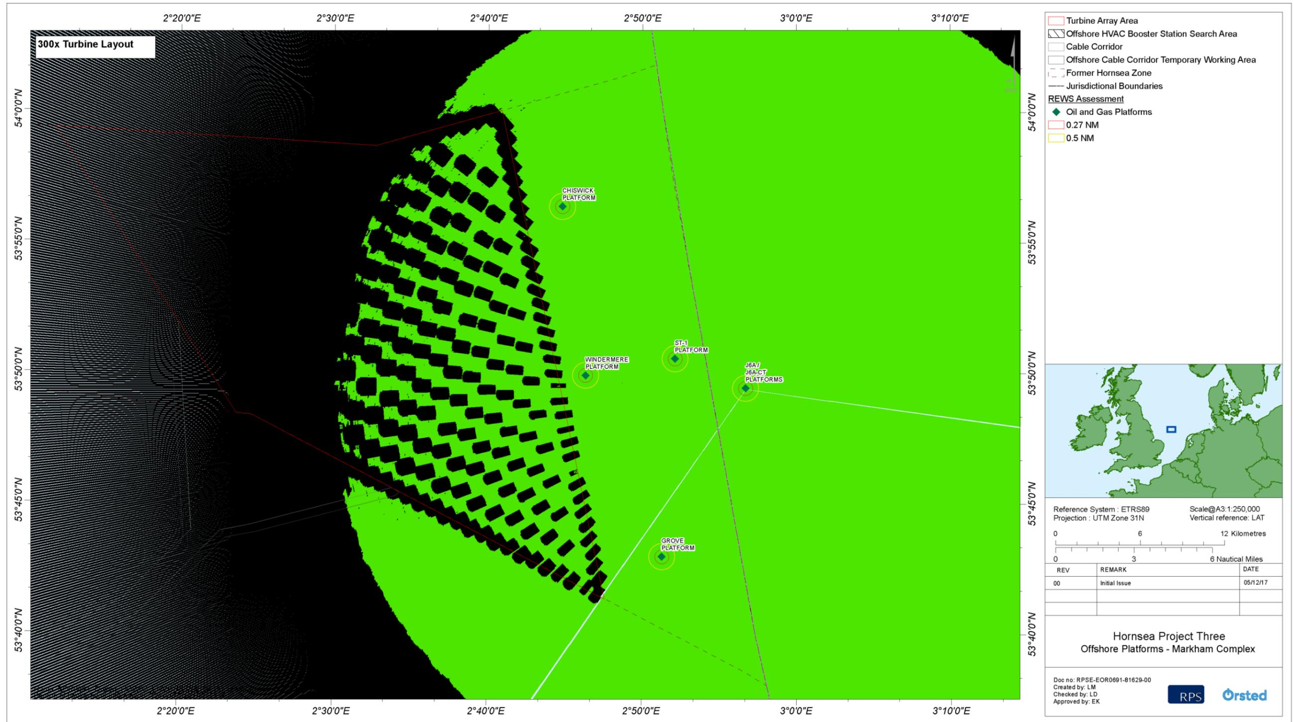
Figure 4.11: J6A platform REWS detection plot showing loss regions for a 100 m<sup>2</sup> target (300 turbines).
