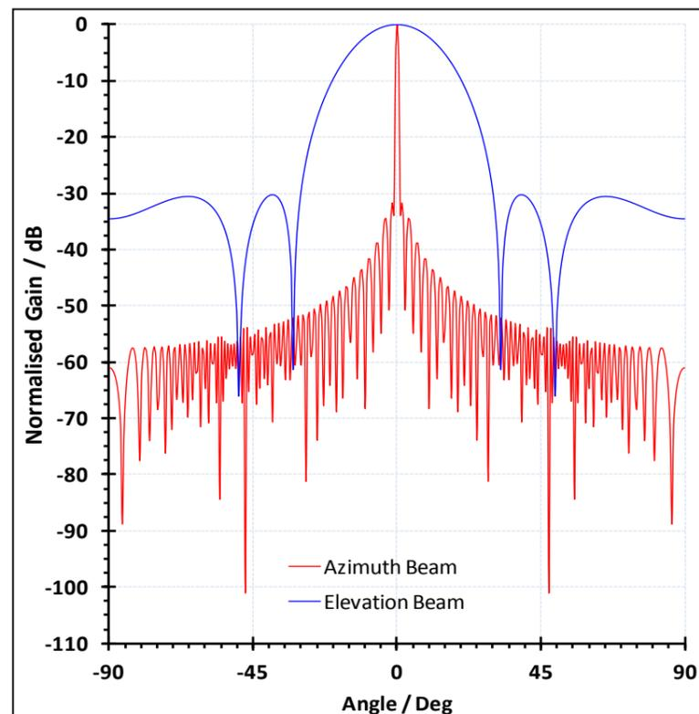
Figure 3.3: The radar antenna elevation and azimuth patterns.
