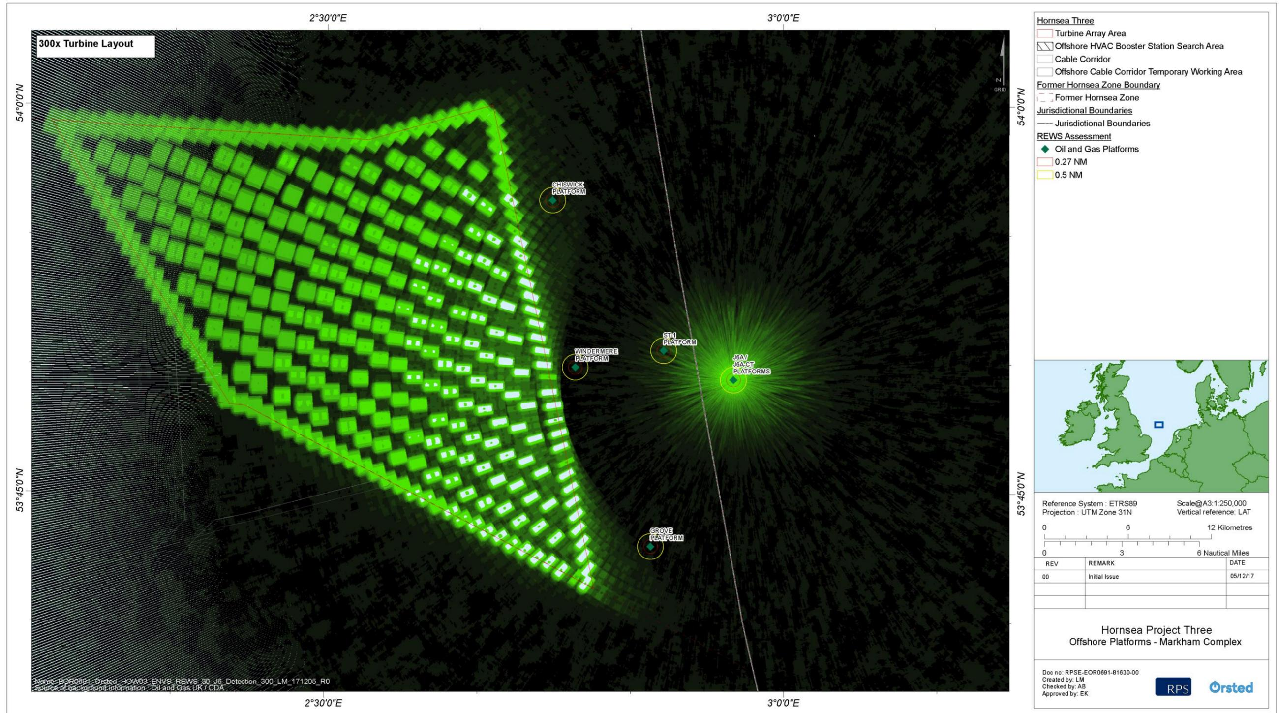
Figure 4.10: J6A platform REWS detection threshold over the Hornsea Three (300 turbines).
