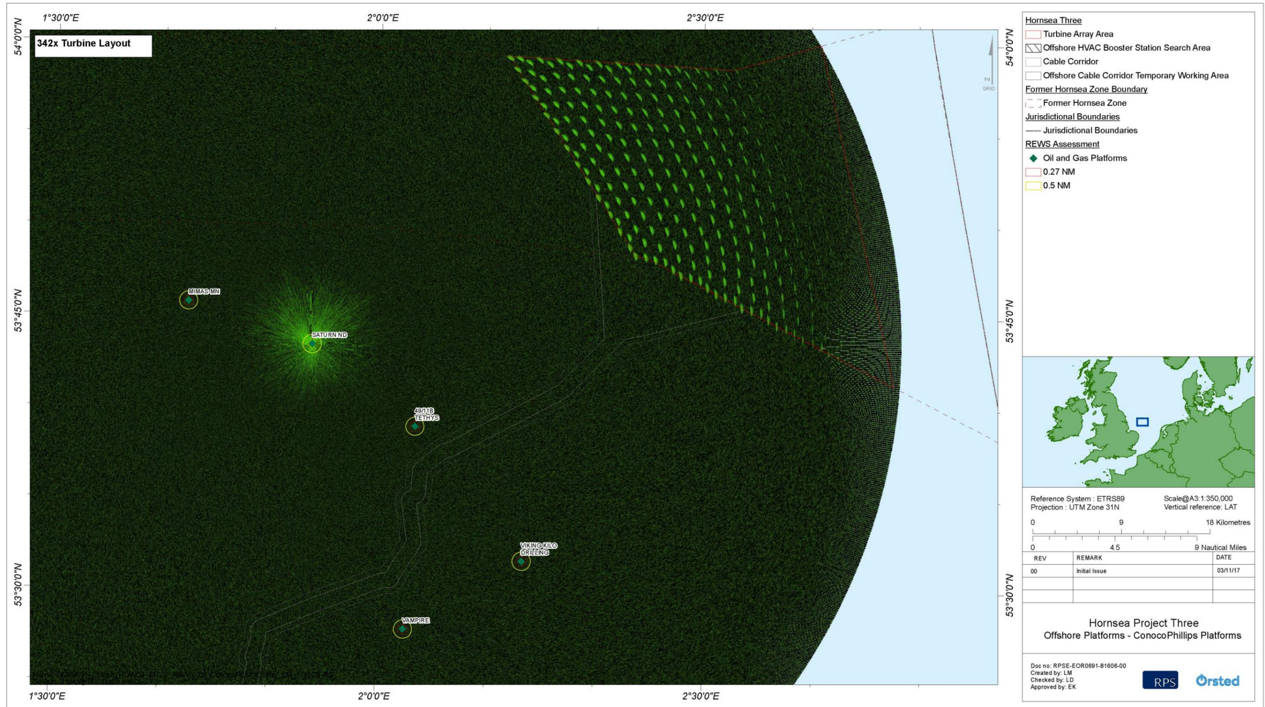
Figure 5.2: Saturn platform REWS clutter map showing returns from Hornsea Three (342 turbines) and sea clutter.
