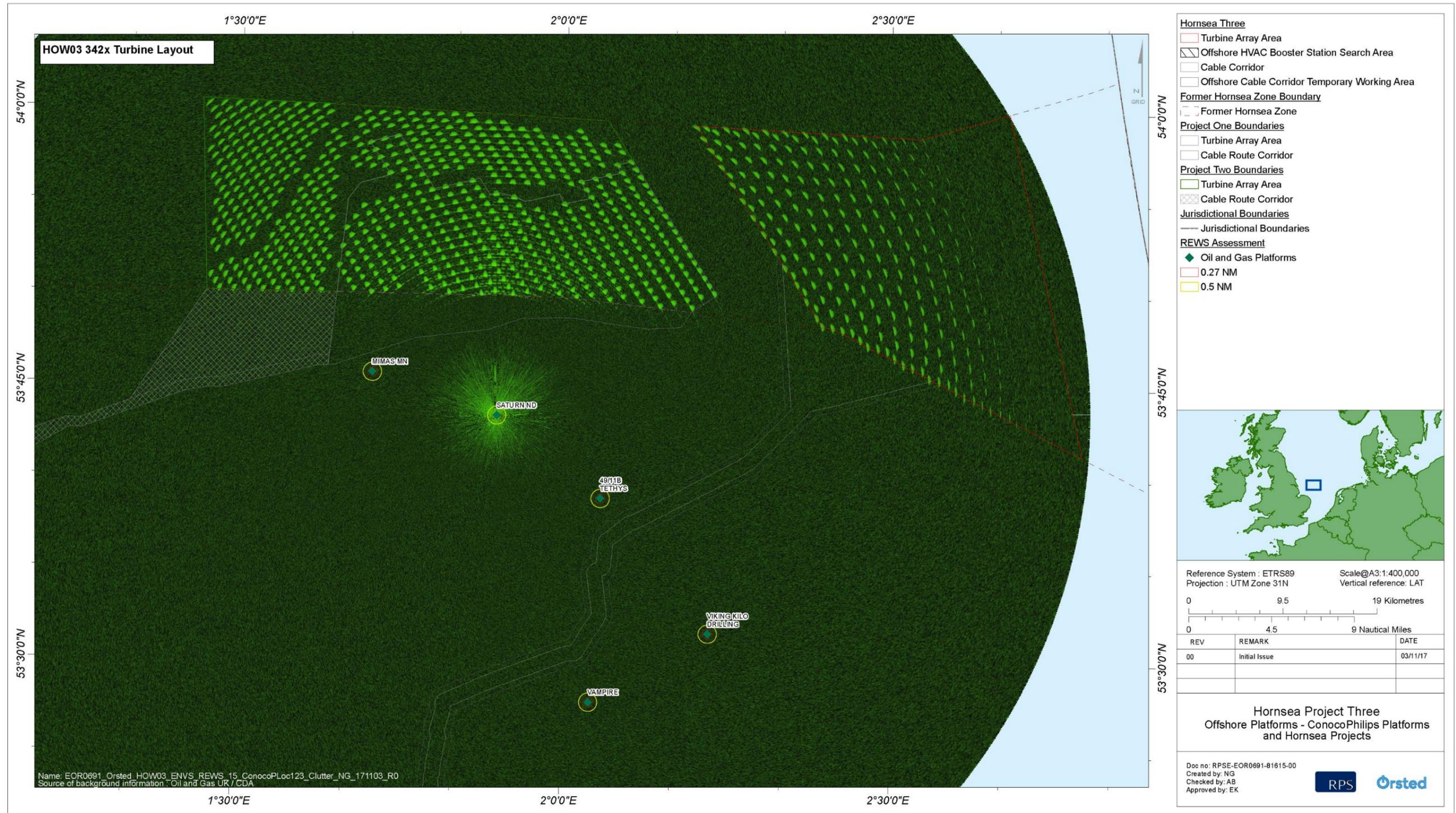
Figure 5.8: Saturn platform REWS clutter map showing returns from the combined Hornsea Project One, Hornsea Project Two and Hornsea Three (342 turbines) and sea clutter. (Note that the Hornsea Project One and Hornsea Project Two consented layouts have less turbines than those shown in this figure).
