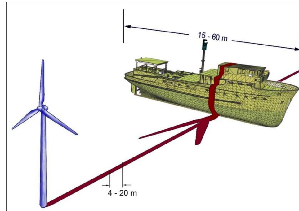
Figure 3.4: Optical blockage and partial shadowing.
