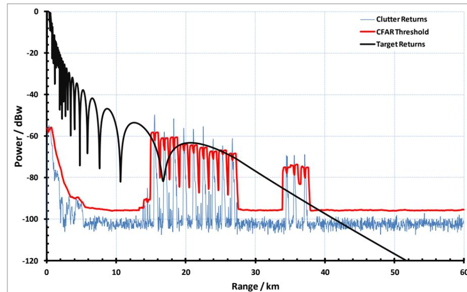
Figure 5.16: Power received from large target at 39° bearing angle.
