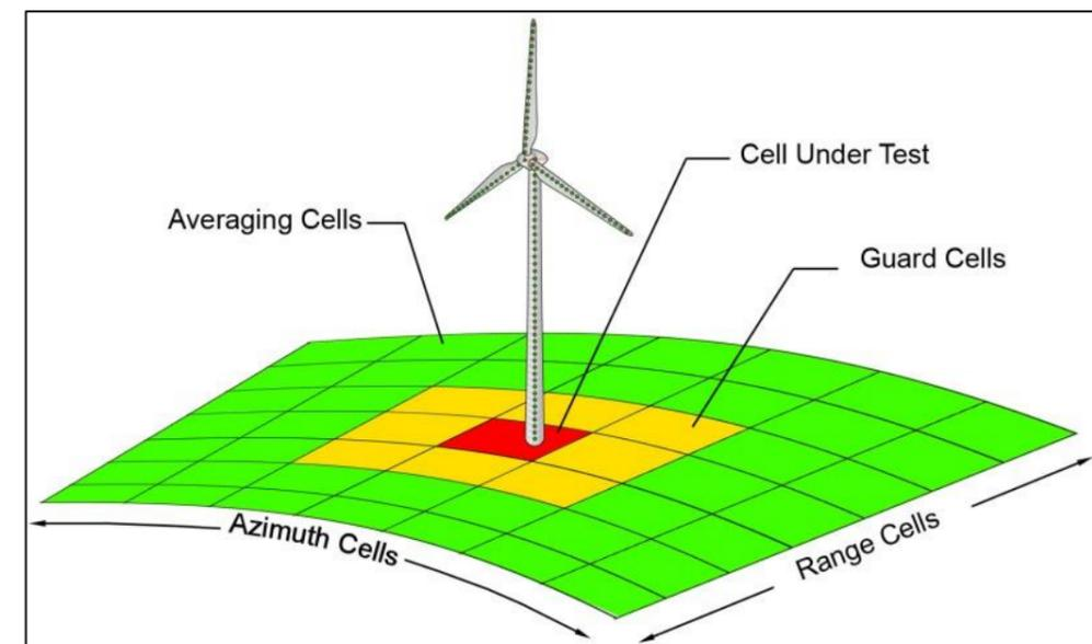
Figure 2.2: 2D CFAR cells around a given cell with wind turbine present.
