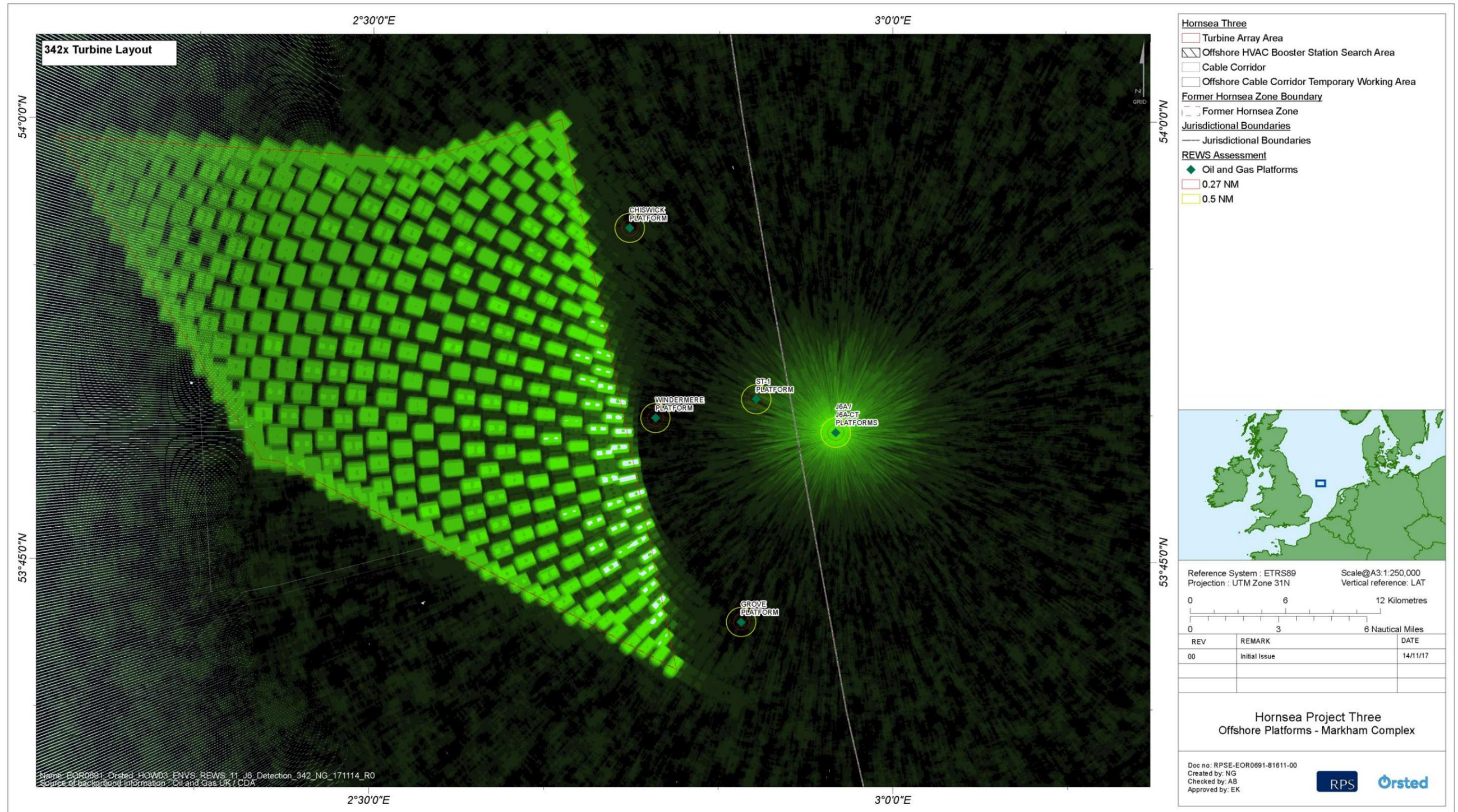
Figure 4.3: J6A platform REWS detection threshold over the Hornsea Three array area (342 turbines).
