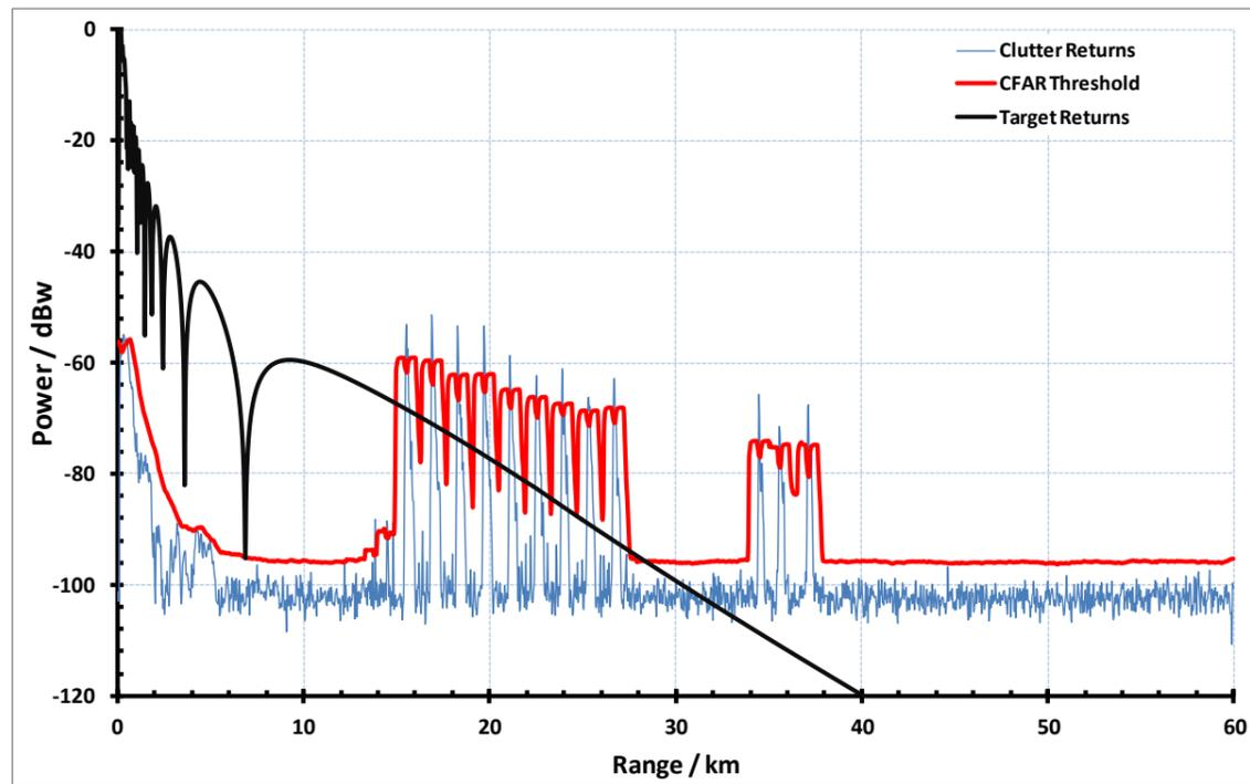
Figure 5.12: Power received from small target at 39° bearing angle.
