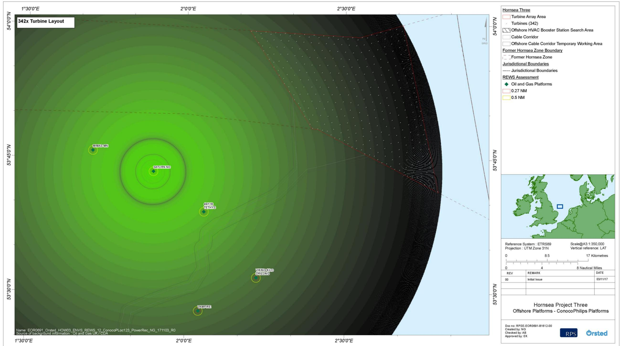
Figure 5.4: Modelled power received from 100 m² target (coverage) (342 turbines).
