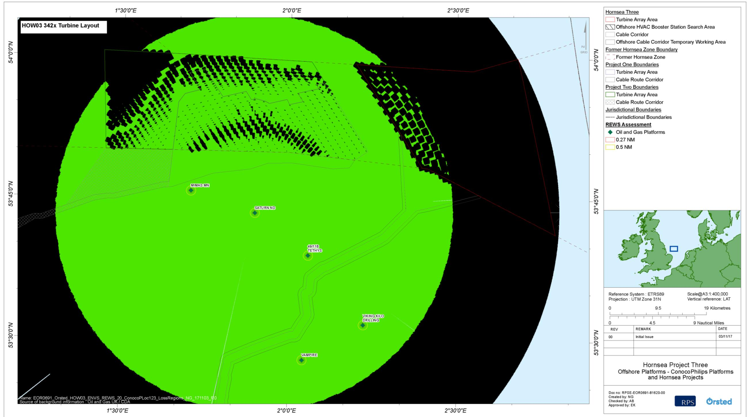
Figure 5.14: Modelled power received from the large 1,000 m<sup>2</sup> target (coverage) (342 turbines). (Note that the Hornsea Project One and Hornsea Project Two consented layouts have less turbines than those shown in this figure).
