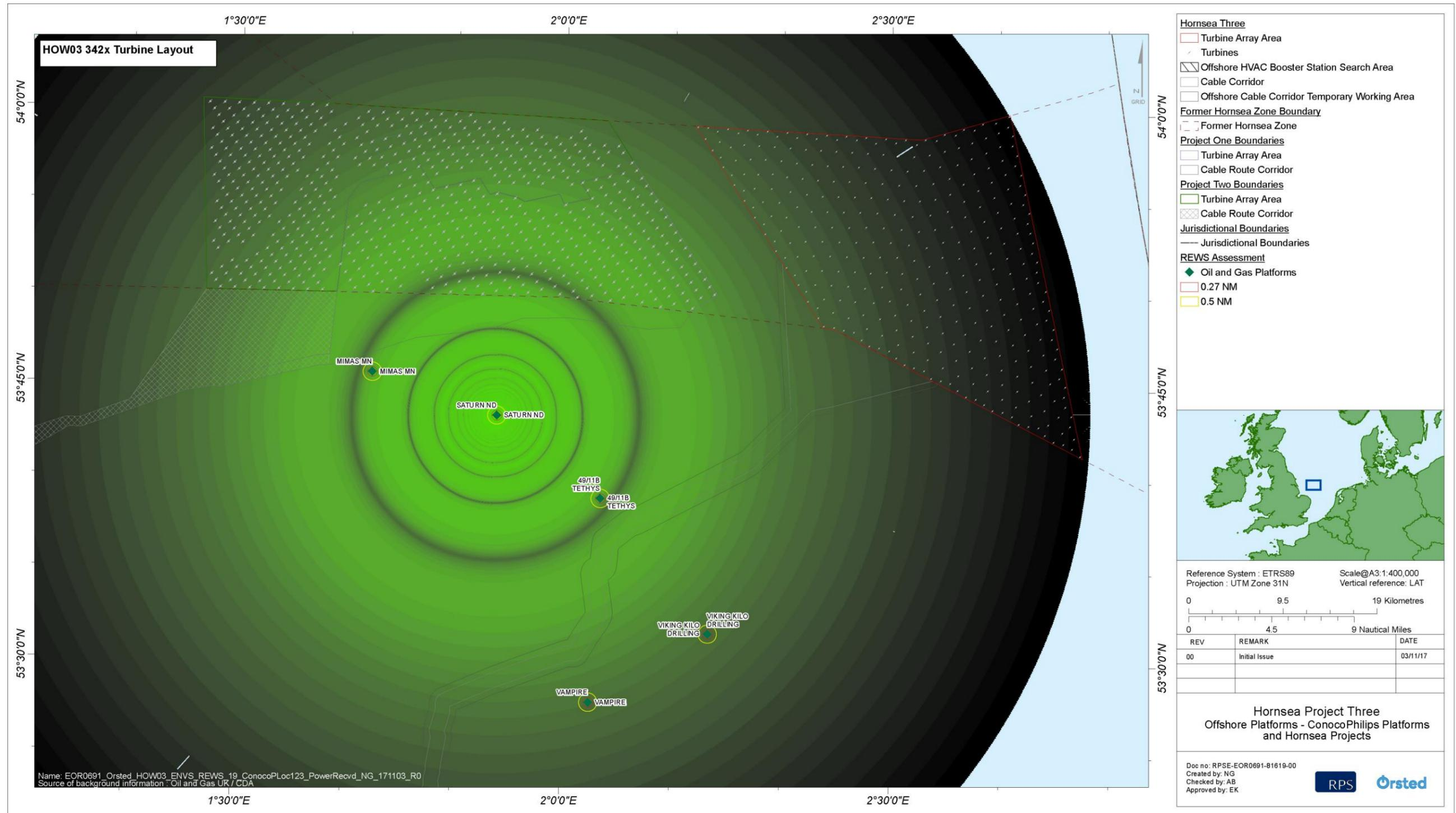
Figure 5.10: Modelled power received from 100 m<sup>2</sup> target (coverage) (342 turbines). (Note that the Hornsea Project One and Hornsea Project Two consented layouts have less turbines than those shown in this figure).
