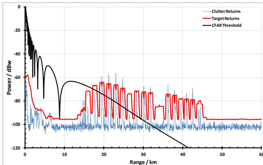
Figure 4.7: Power received from small target at 283° bearing angle.
