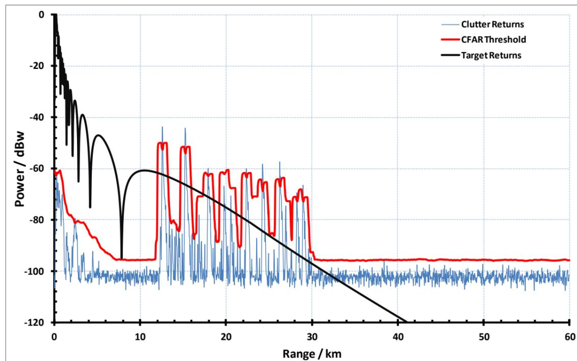
Figure 5.13: Power received from small target at 0° bearing angle.
