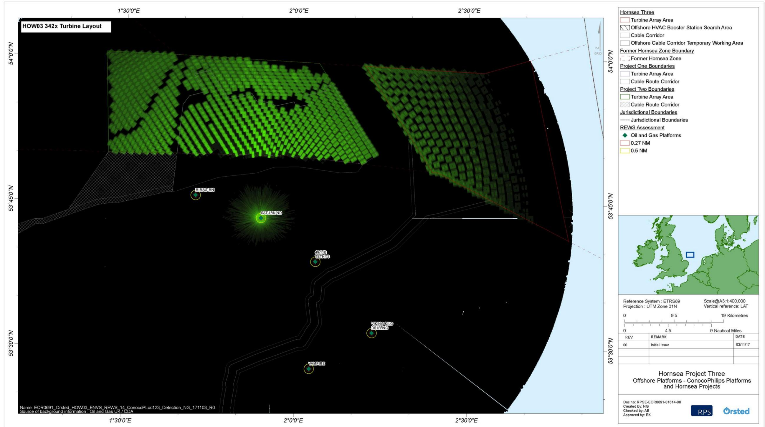
Figure 5.9: Saturn platform REWS detection threshold over the combined Hornsea Project One, Hornsea Project Two and Hornsea Three (342 turbines). (Note that the Hornsea Project One and Hornsea Project Two consented layouts have less turbines than those shown in this figure).
