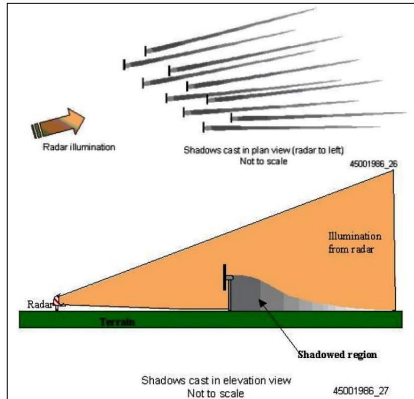
Figure 2.1: Illustration of radar shadowing with diffraction effects (Butler and Johnson, 2003).
