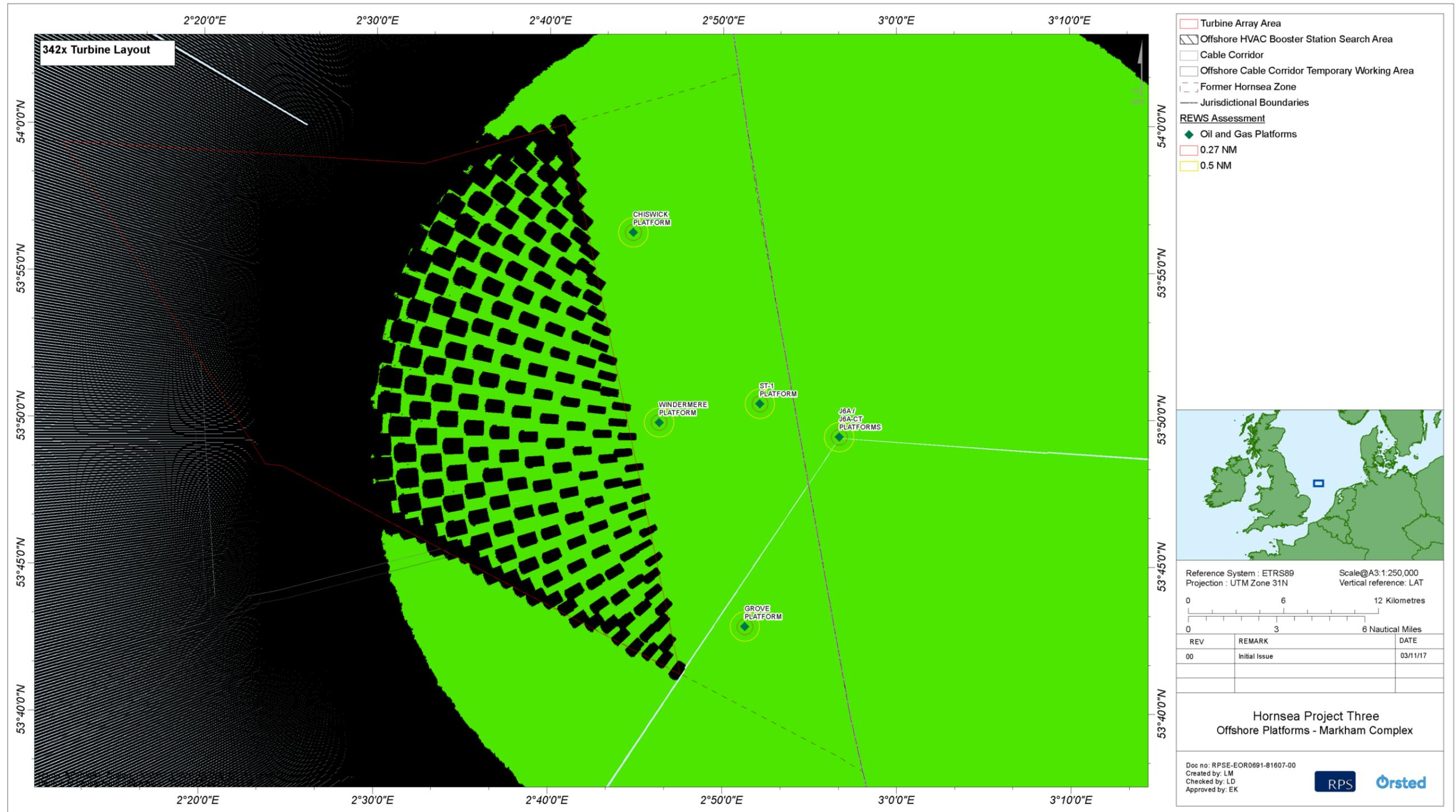
Figure 4.5: J6A platform REWS detection plot showing loss regions for a 100 m<sup>2</sup> target.
