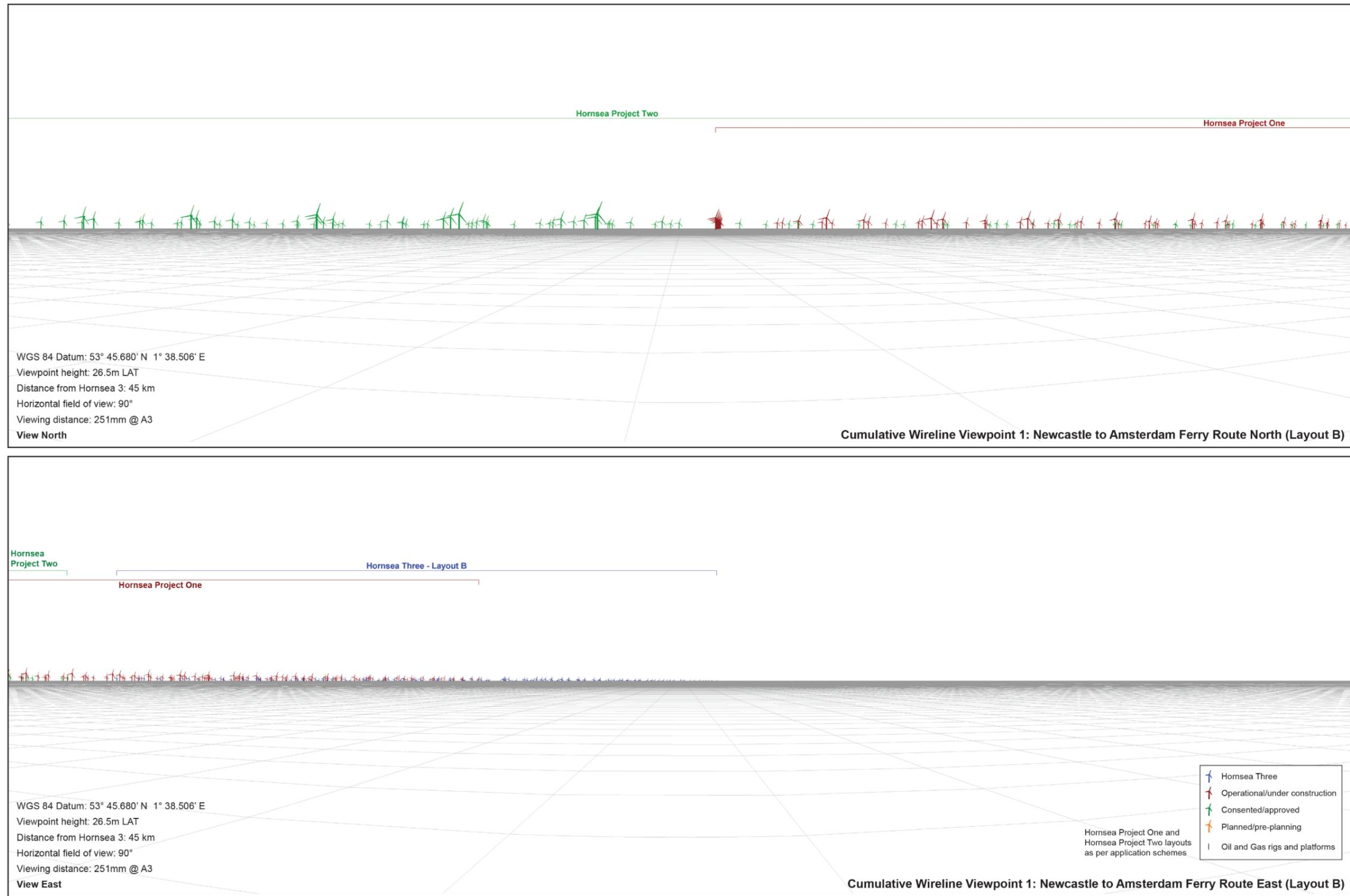
Figure 8: Cumulative wireline viewpoint 1: Newcastle to Amsterdam ferry route north and east (Layout B - 160 turbines with a maximum blade tip height of 325 m).
