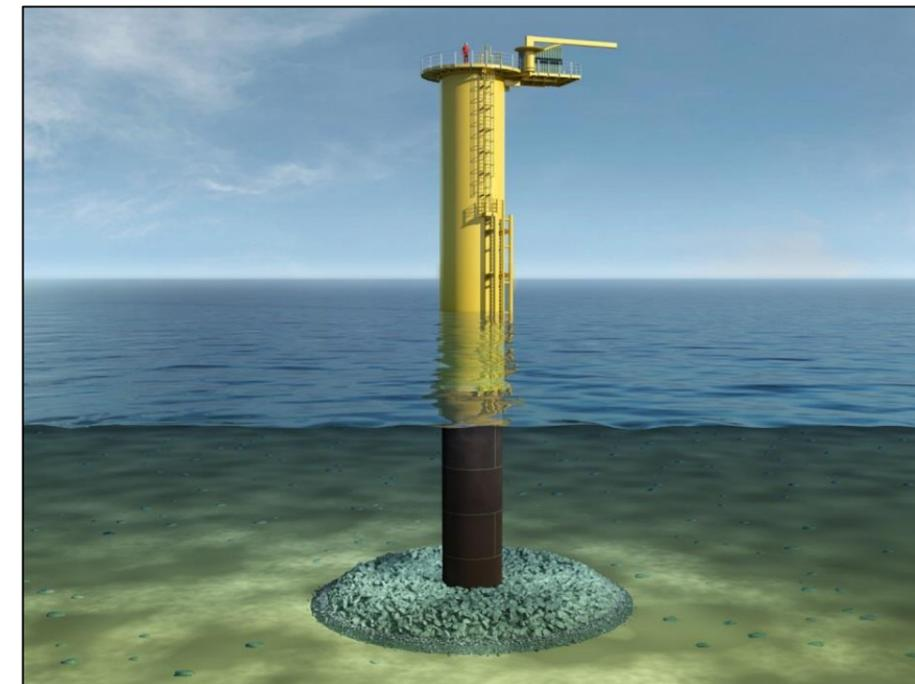
Figure 3.11: A monopile foundation and transition piece.
