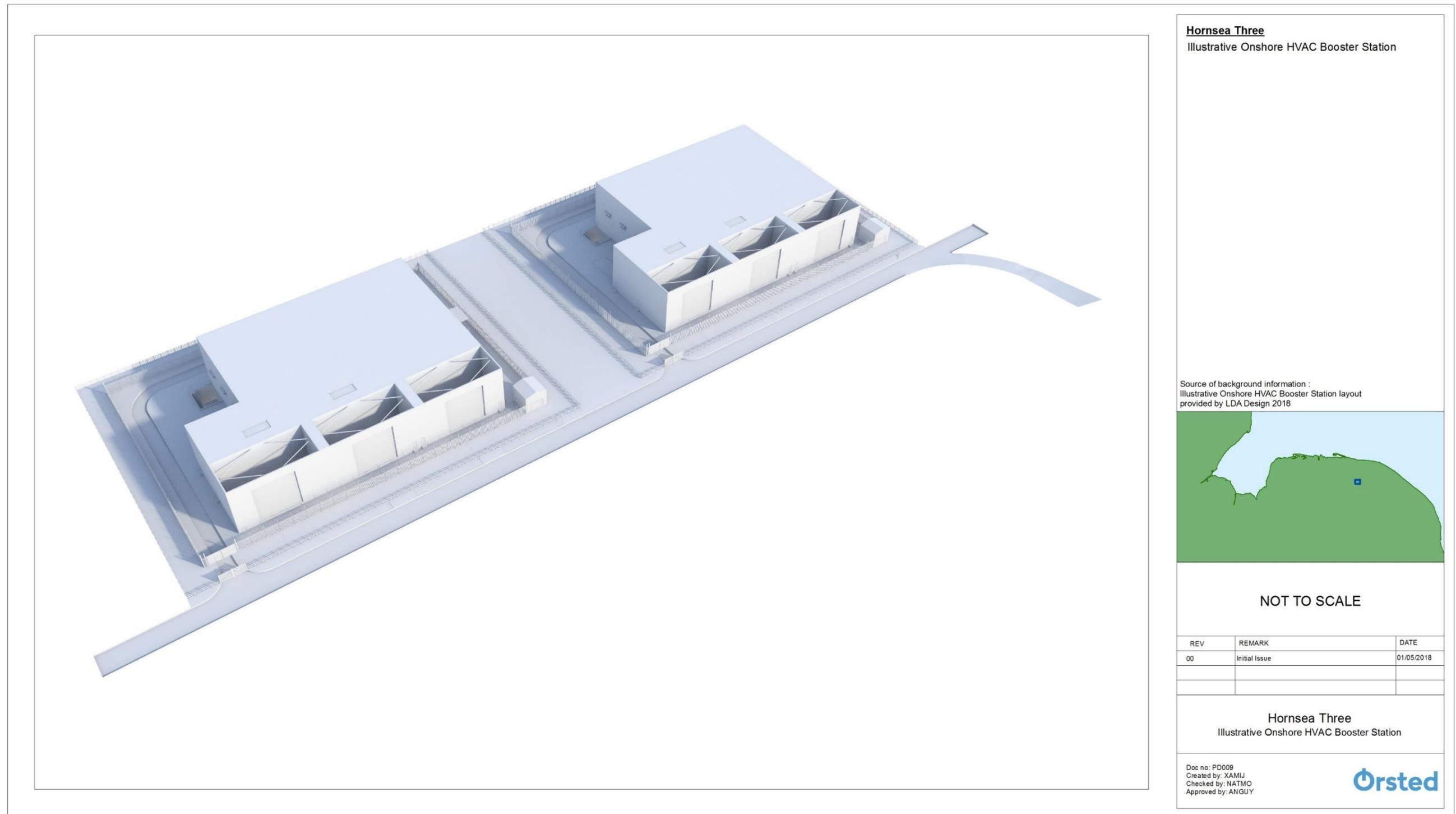
Figure 3.34: Indicative onshore HVAC booster station layout .
