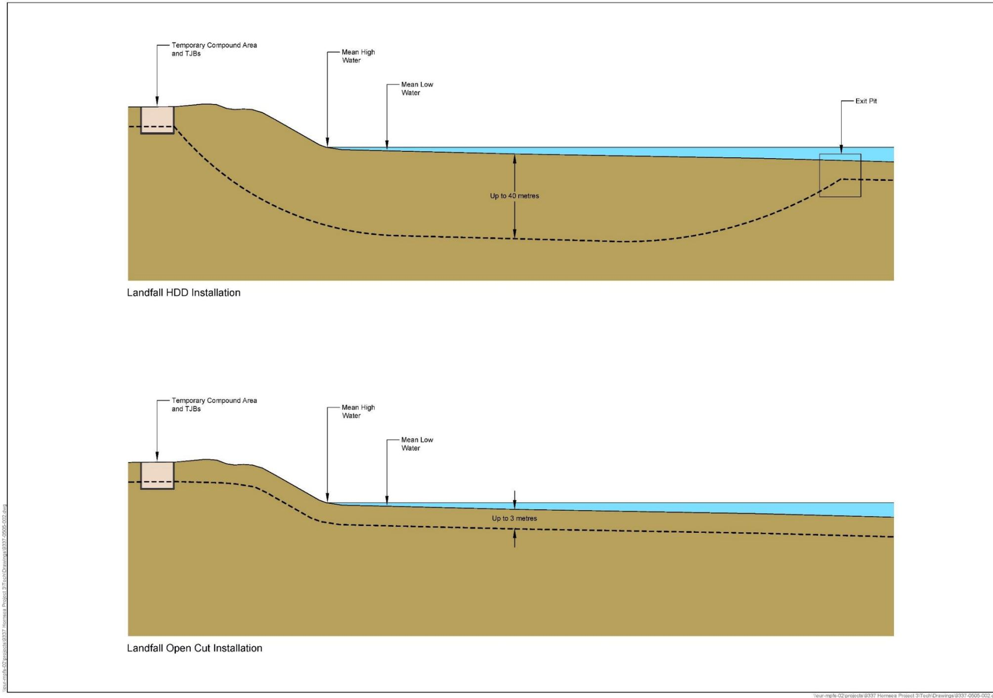
Figure 3.22: Indicative HDD and open cut arrangement.
