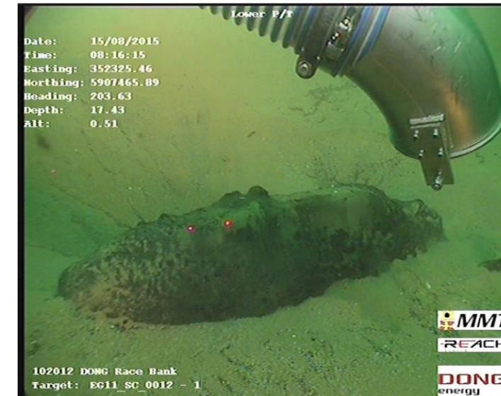
Figure 3.3: An example of a UXO following excavation.
