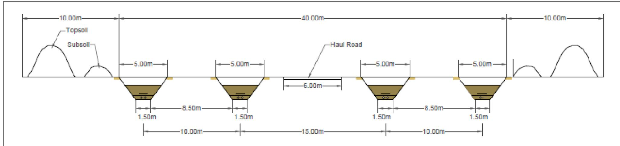
Figure 3.36: Grid connection export cable corridor indicative layout.
