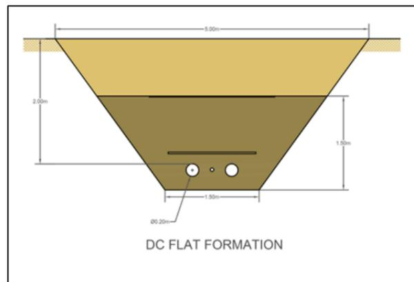
Figure 3.31: Onshore export cable HVDC trench layout.
