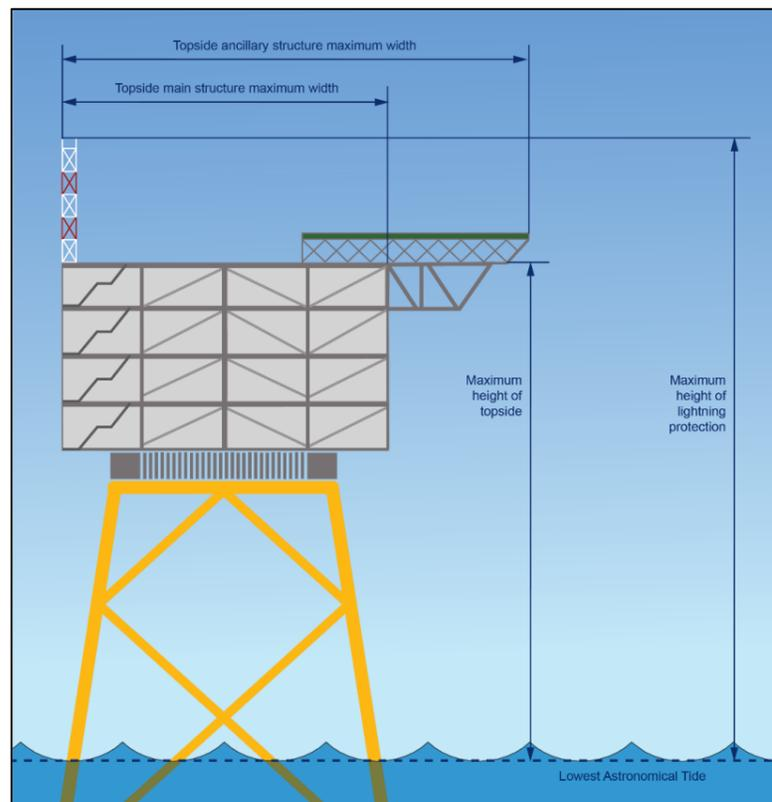
Figure 3.18: Schematic of an offshore transformer substation.
