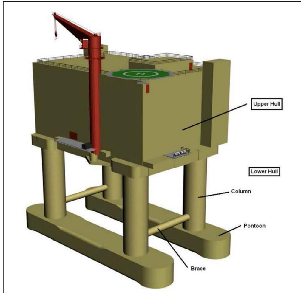
Figure 3.14: An example of a converter substation design supported by a pontoon gravity base – type 1<sup>1</sup> foundation.
