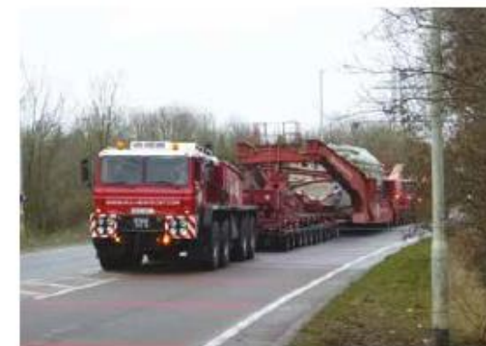
Specialist trucks arriving with transformers at Walney Extension Offshore Wind Farm.
