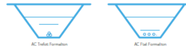
Onshore export cable HVAC trench layouts.
