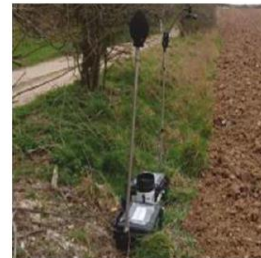
Noise monitoring equipment.
