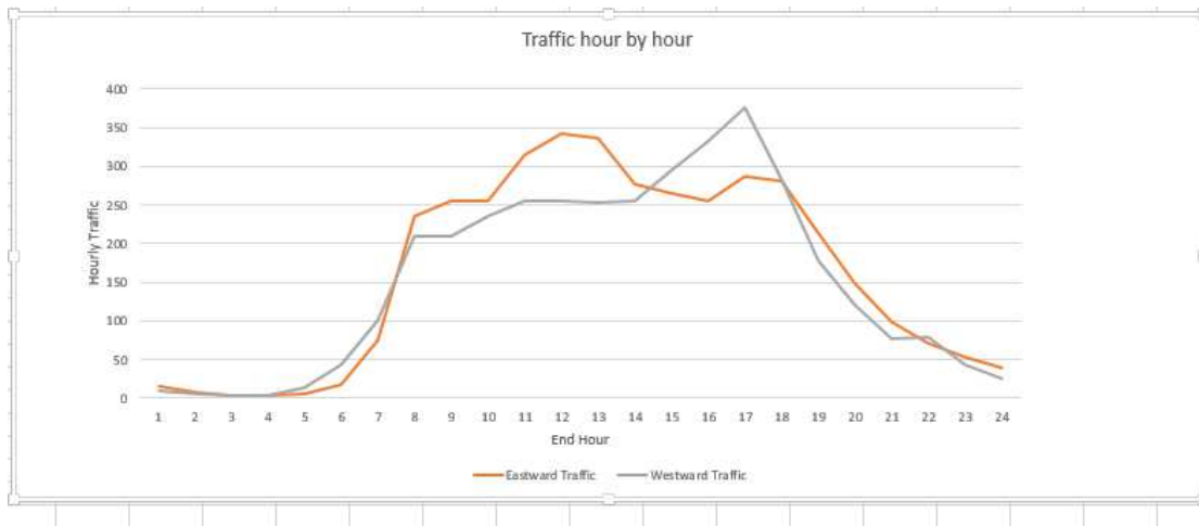
Figure 2: Average traffic count along the A1094 hour by hour garnered by SPR
