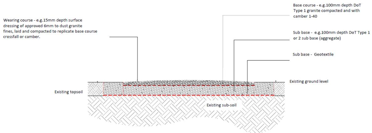
Public Right of Way - Aggregate path surfacing specification
