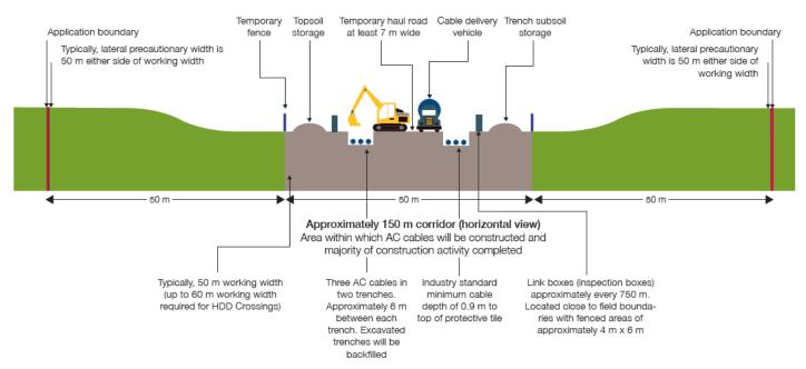
This illustration is for illustrative purposes only and is intended to show the typical construction of AC cables for interconnectors in the UK
