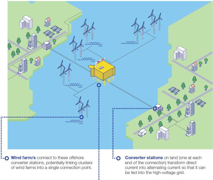
An offshore converter station transforms the alternating current into direct current, enabling it to pass through the HVDC cable.
