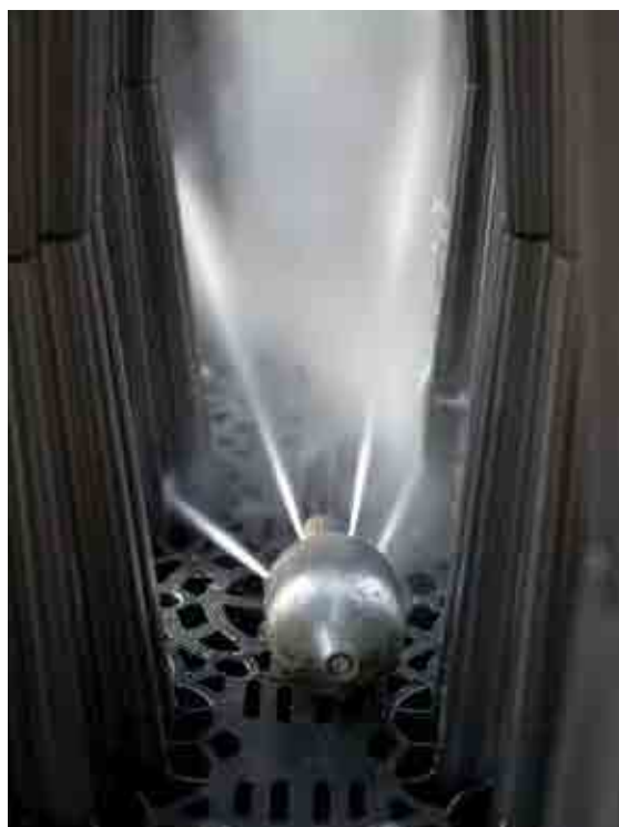
Figure 21.19 Some system configurations allow jetting equipment to move within the structure (courtesy ACO Limited)
