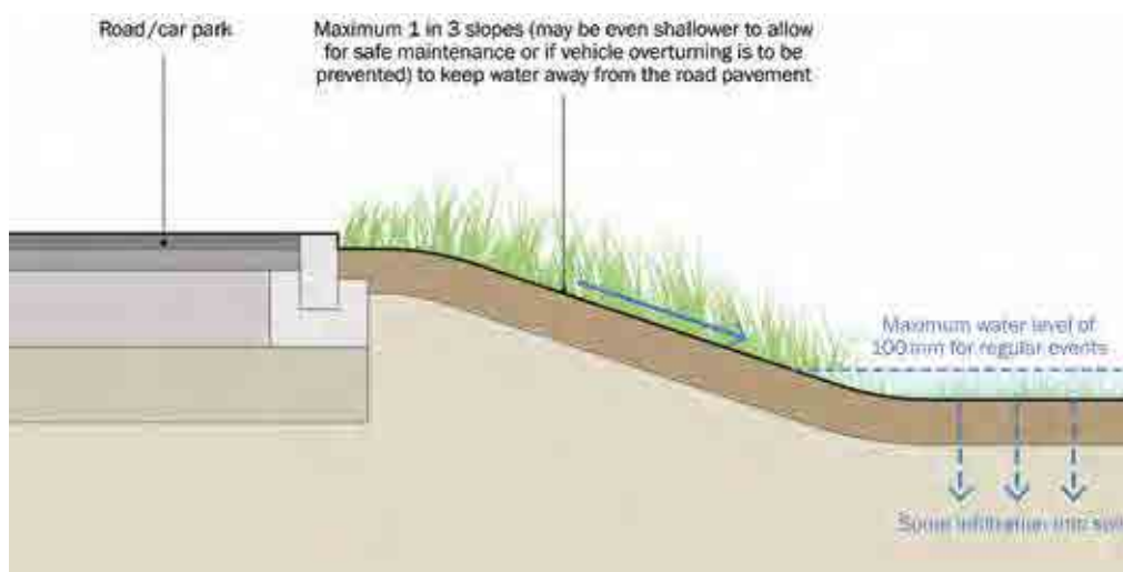
Figure 9.13 Water flows from shallow swales acting as edge drains for the road sub-base
