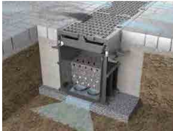
Outflow is via a perforated pipe in the filter media (courtesy Stormwater Management and Funke Kunststoffe GmbH)
