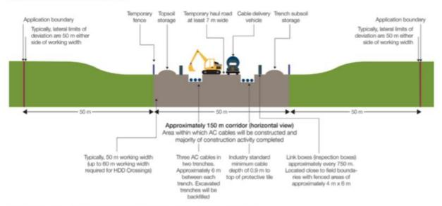
This Bustration is for Bustrative purposes only and is intended to show the typical construction of AC cables for interconnectors in the UK
