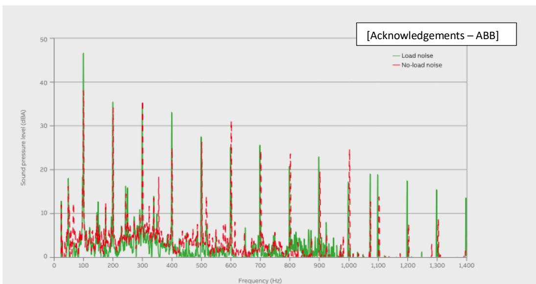
(FFT showing HVAC Sound Pressure Levels as function of frequency)
