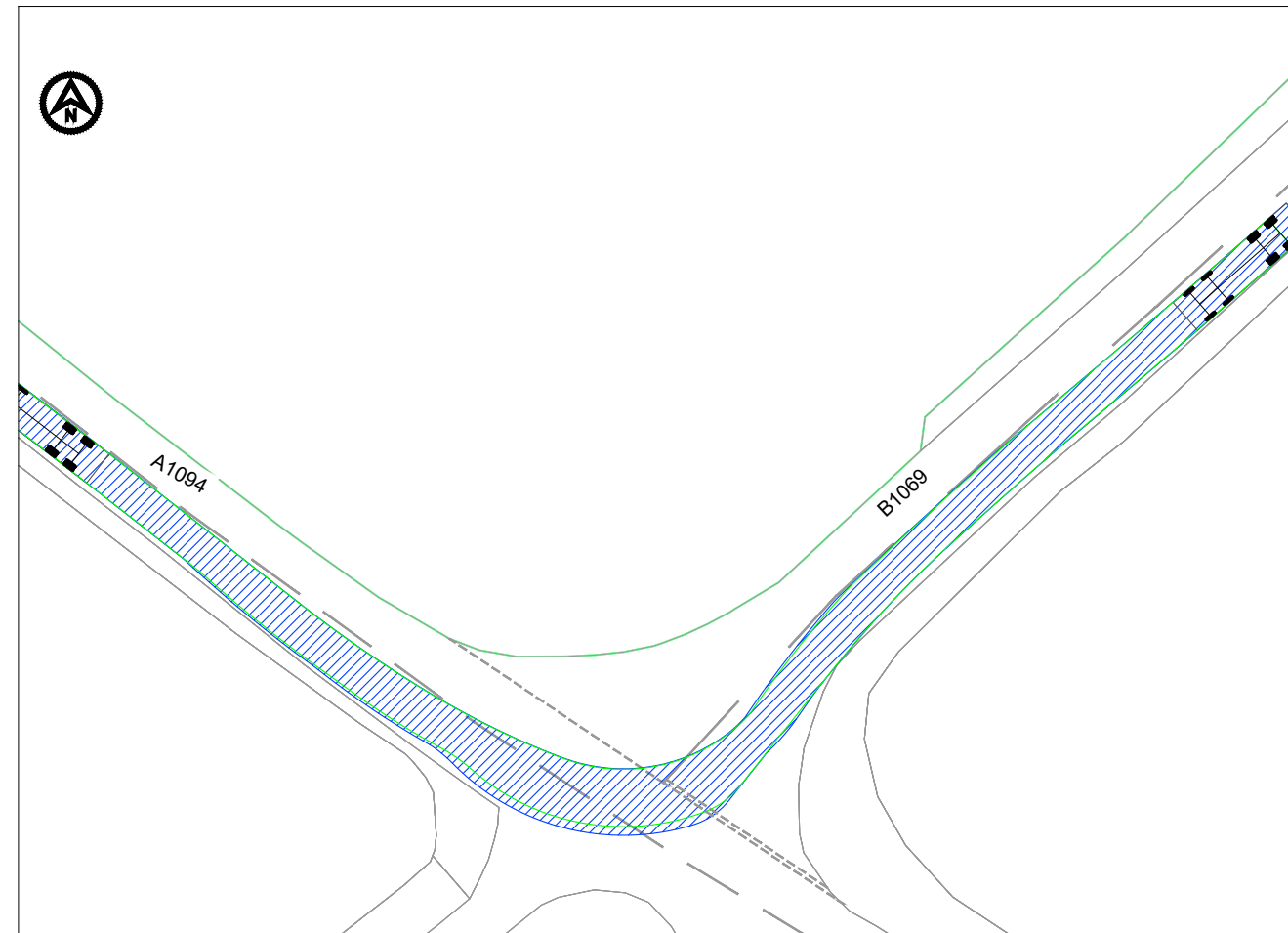
LARGE TIPPER TURNING BETWEEN A1094 TO B1069
