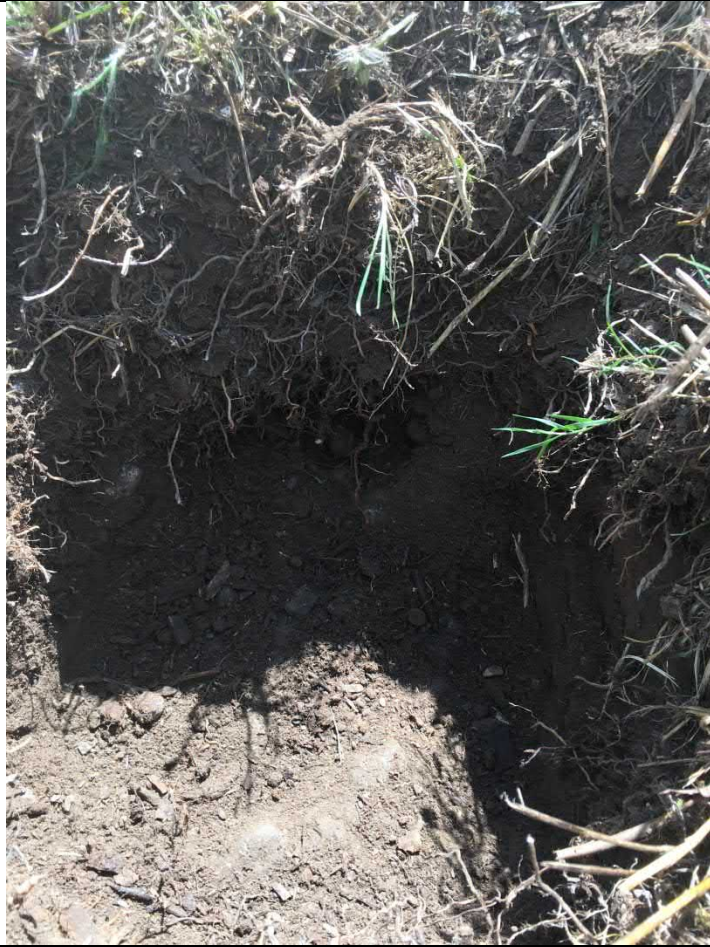
Photograph 13: TP23 showing succession of glacial deposits including compacted boulders underlying topsoil
