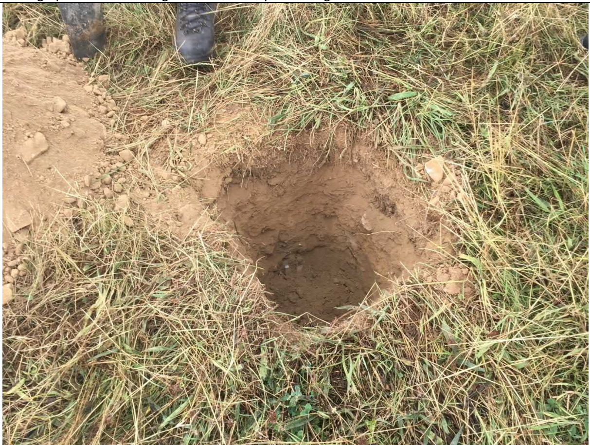
Photograph 2: TP46 showing glacial deposits beneath topsoil
