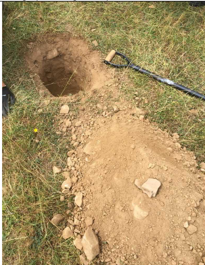
Photograph 4: TP43 sandy gravelly clay with medium cobble content
