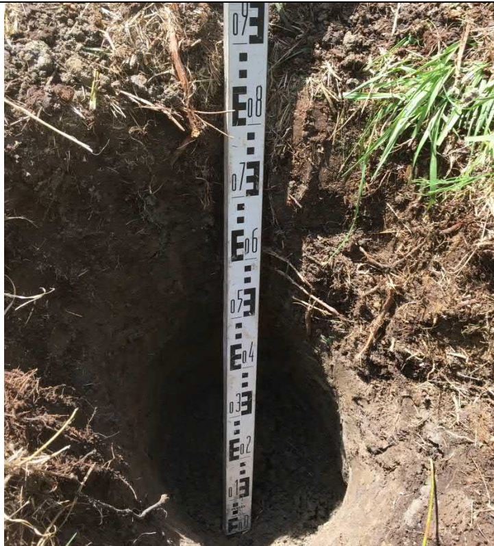
Photograph 14: TP24 showing succession of topsoil over glacial deposits
