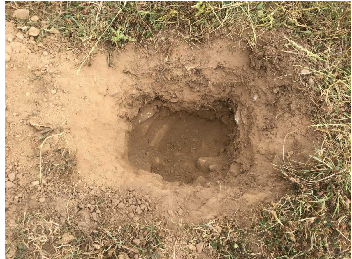
Photograph 7: TP36 showing glacial deposits with impassable boulders at base of pit
