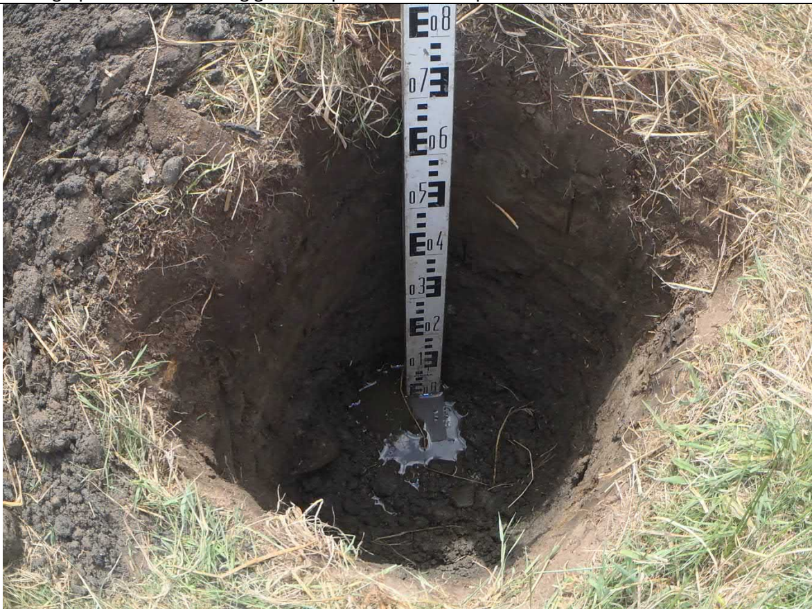
Photograph 22: TP17 showing topsoil over glacial deposits. Water ingress at base associated with gravel band
