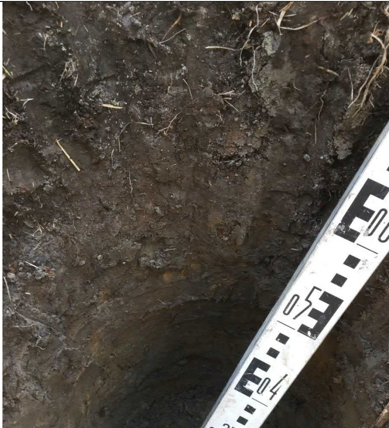
Photograph 15: Detail of clayey topsoil with many rootlets in TP24
