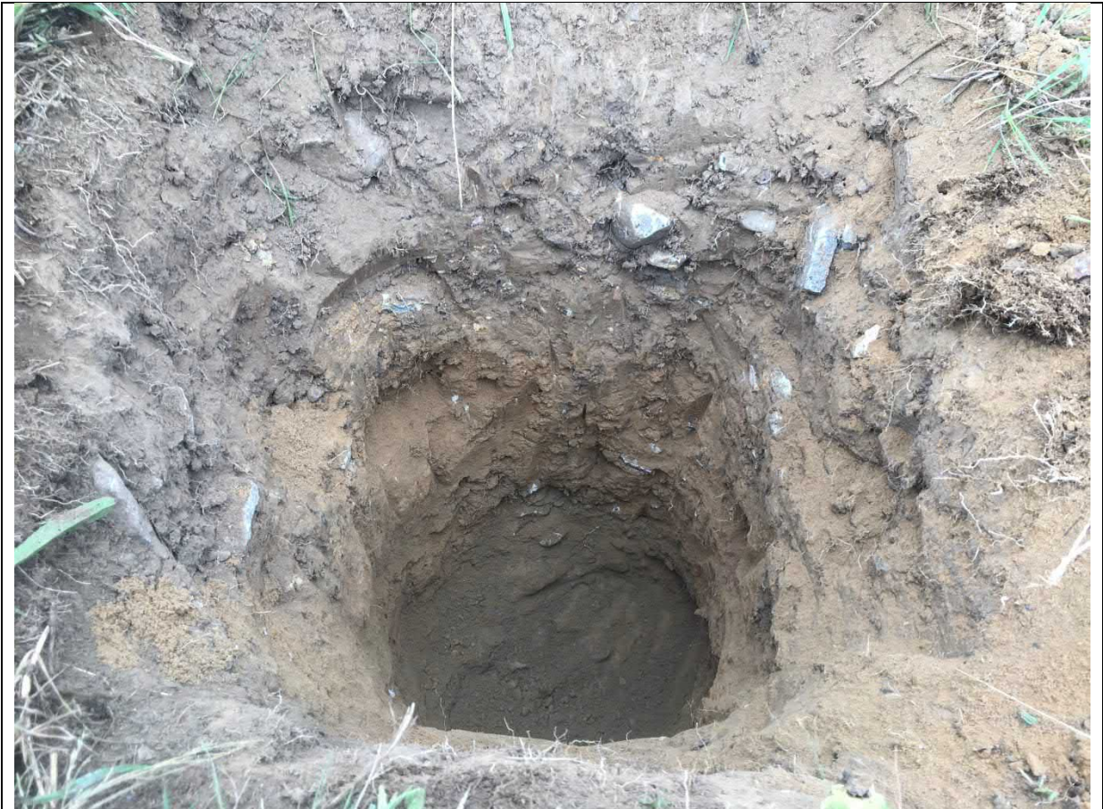
Photograph 3: TP45 showing topsoil over glacial deposits
