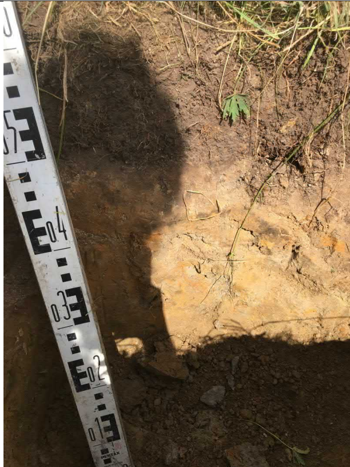
Photograph 18: TP21 showing succession of topsoil over glacial deposits
