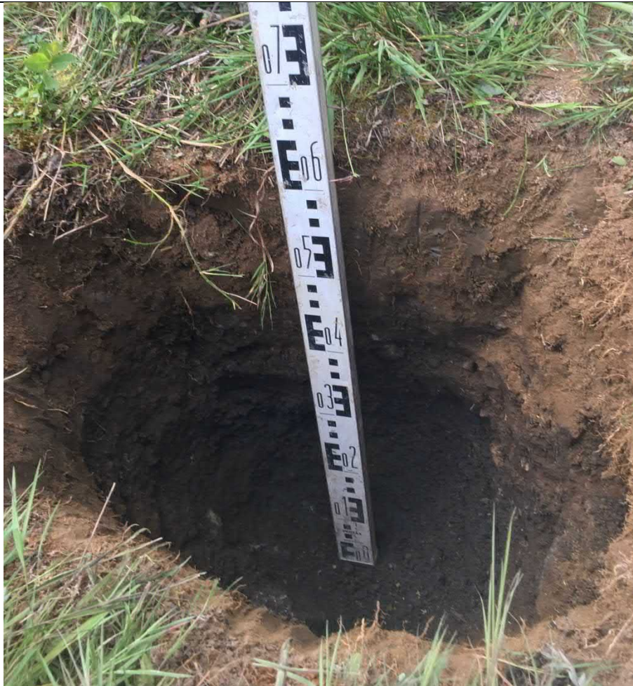
Photograph 11: TP25a showing made ground deposits
