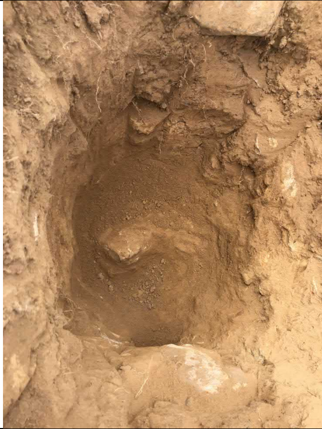
Photograph 5: Base of TP43 showing impassable boulder
