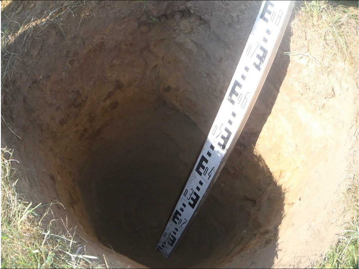
Photograph 21: TP20 showing glacial deposits beneath topsoil
