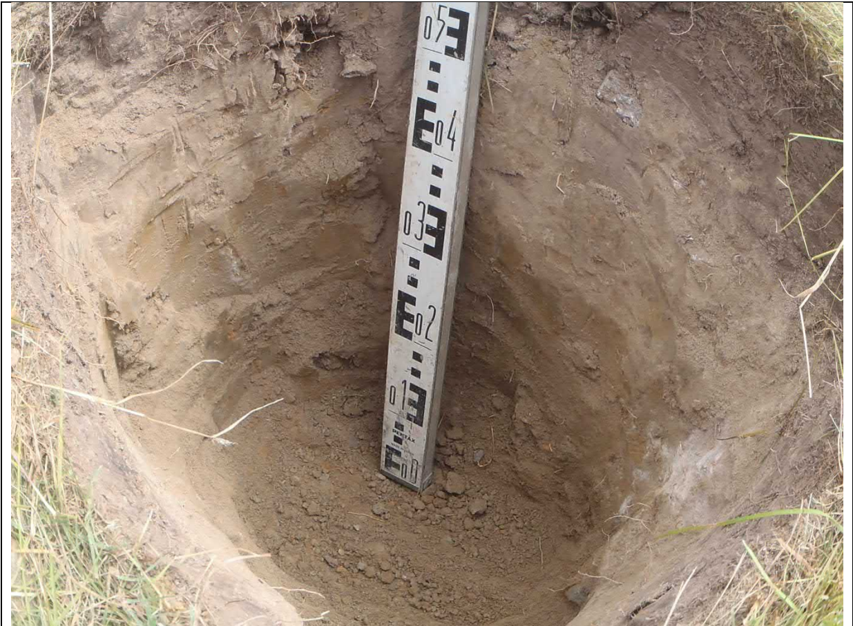
Photograph 23: TP31 showing glacial deposits comprising slightly gravelly sandy clay with low cobble content
