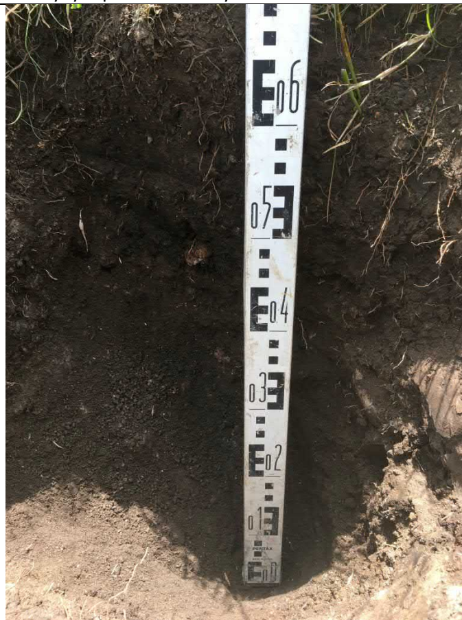
Photograph 16: TP22 showing succession of topsoil over made ground with glacial deposits at base
