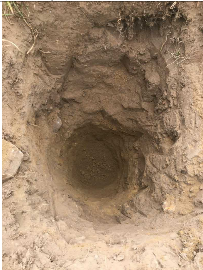
Photograph 6: TP41 showing succession of topsoil over glacial deposits
