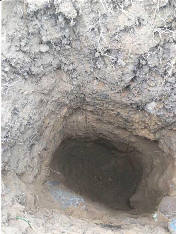
Photograph 1: TP47 showing succession of topsoil over glacial strata
