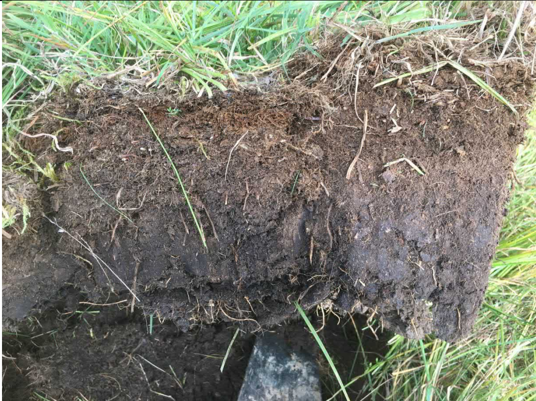
Photograph 19: TP16 sandy clayey topsoil with frequent rootlets overlying glacial deposits
