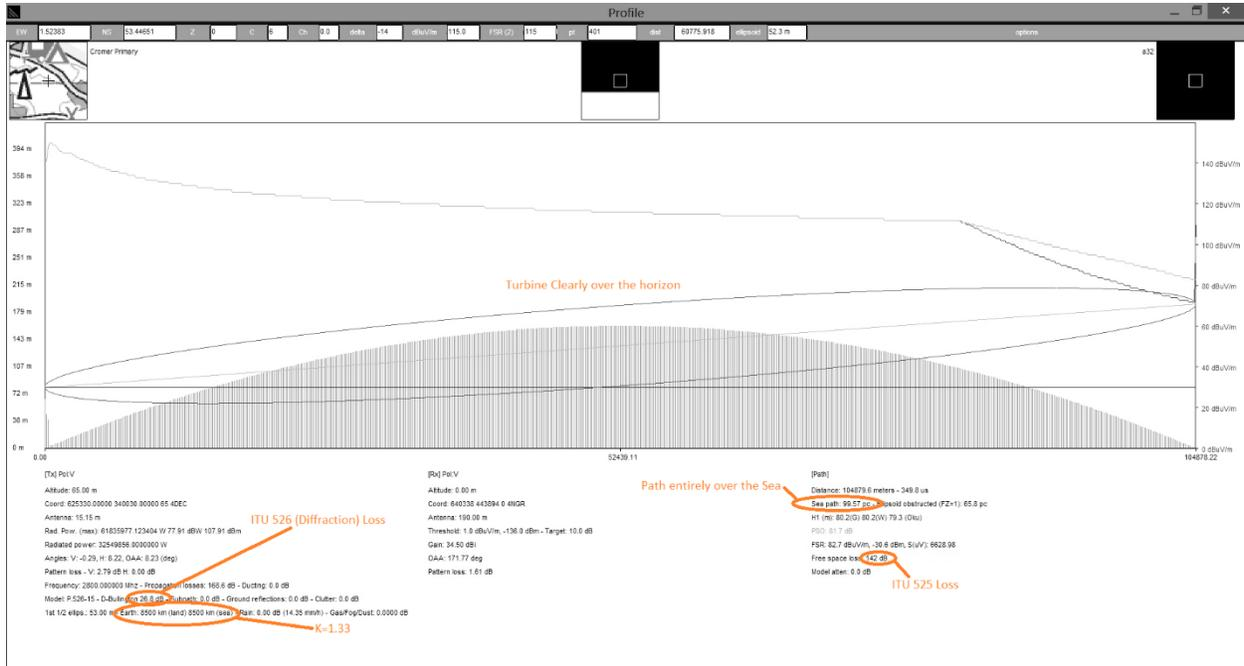
The software was then used to simulate losses over the same path at various time percentages using an ITU 452 based methodology.
