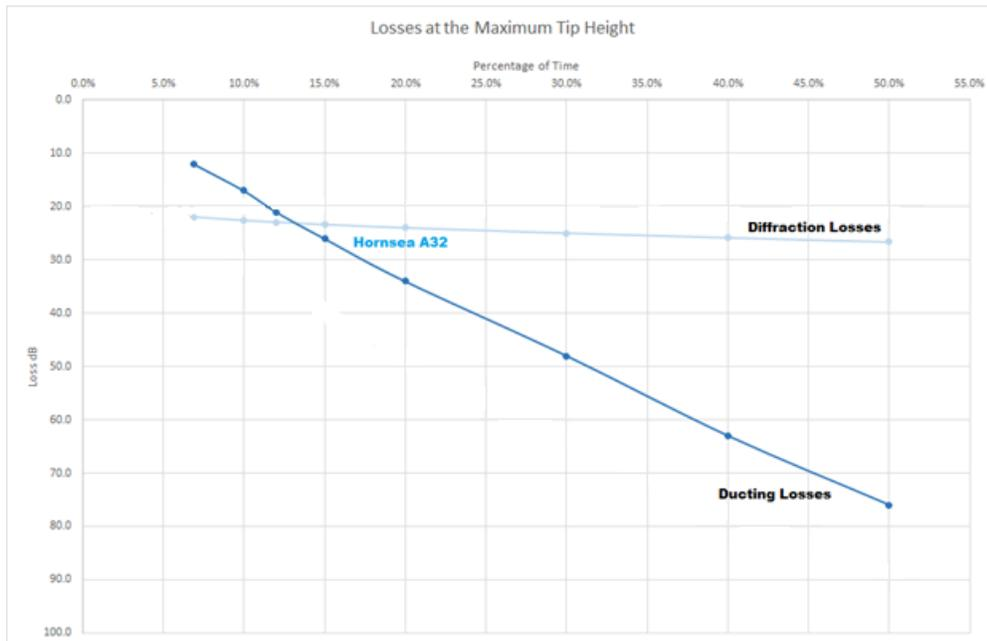
As expected, the 27dB figure for the median day (diffraction being the dominant mode at 50%) aligns with the predicted ITU 526 losses. As the time percentage parameter reduces this does not vary much
