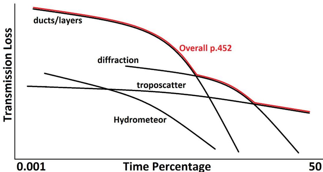
For radar-turbine assessments, troposcatter is not a significant factor. The current methodology, therefore, based solely on diffraction, aligns with the recommendation for the median day. For the proportion of time where ducts/layers become the dominant mode it is likely to significantly overestimate the losses and therefore underestimate the probability of detection.
