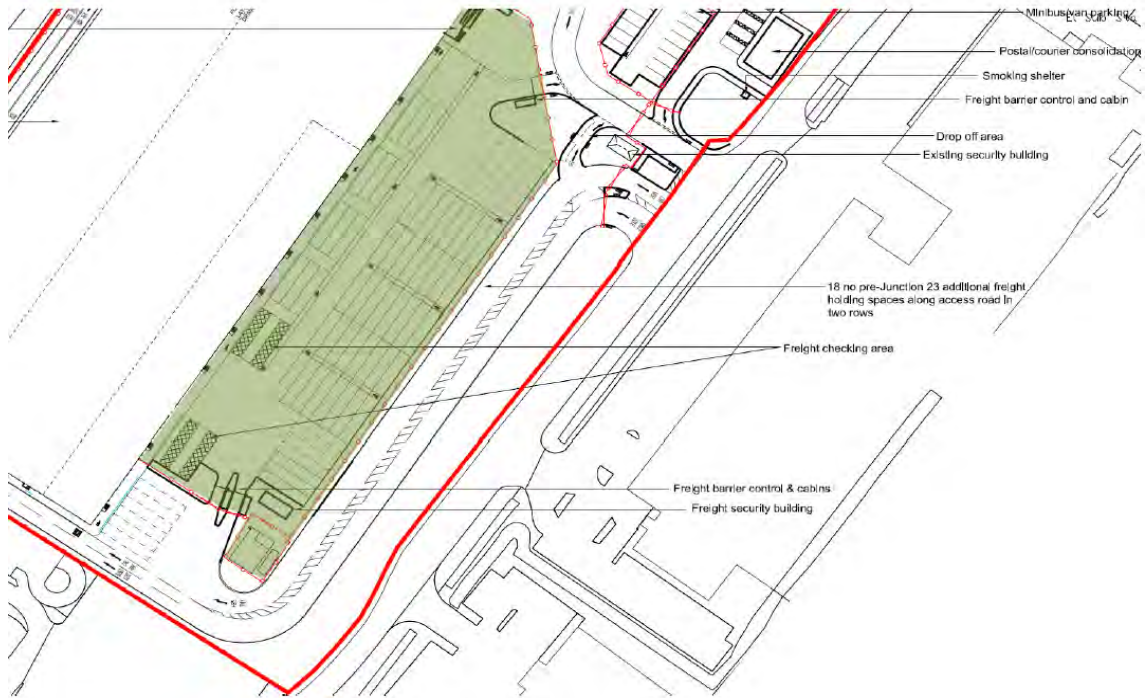
Figure 6.11: Layout of Freight Management Facility at Junction 24
