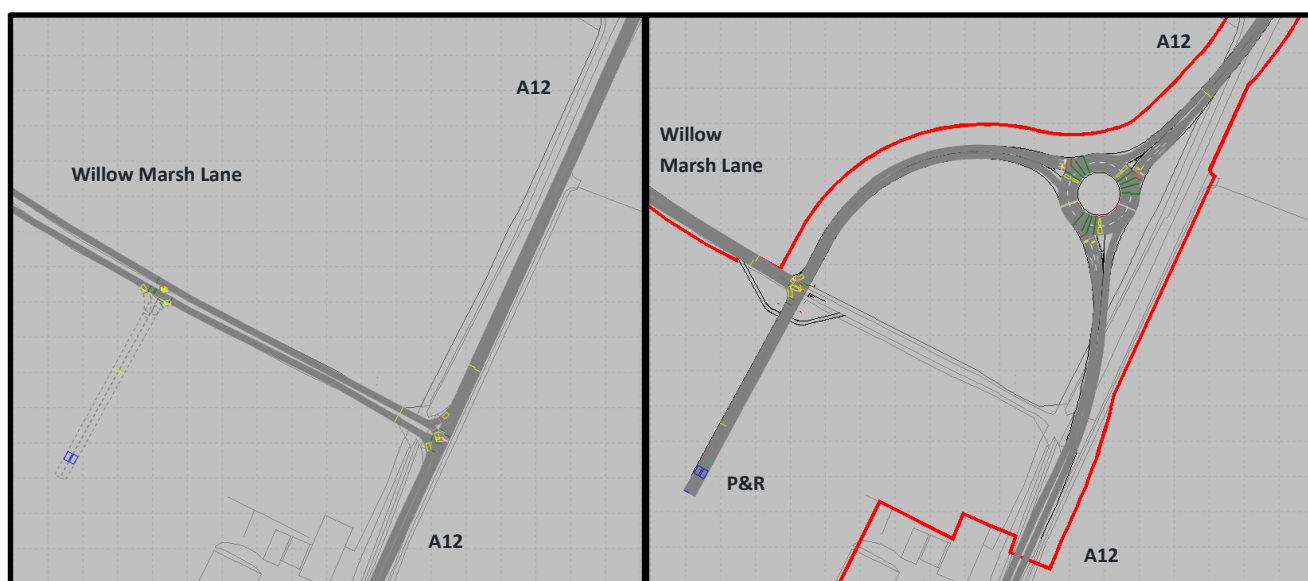
Figure 36 – Northern park and ride site access before and after construction
