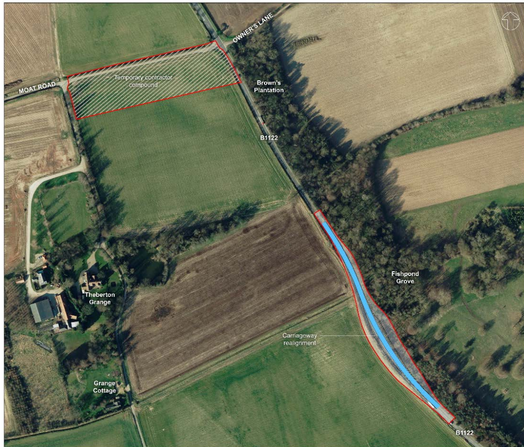
Plate 9.7: Improvement to the alignment of the B1122 between Theberton and the Sizewell C construction site entrance.
