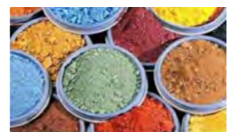
Concrete colour can be influenced by pigmentation addition
