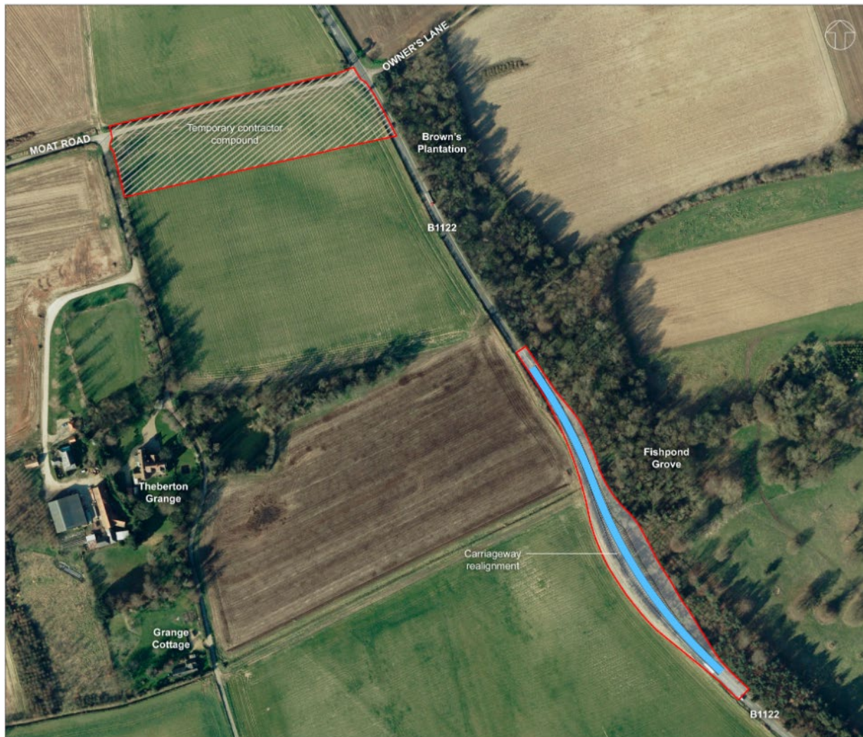
Plate 3.4: Stage 2 – Improvement to the alignment of the B1122 between Theberton and the Sizewell C construction site entrance.
