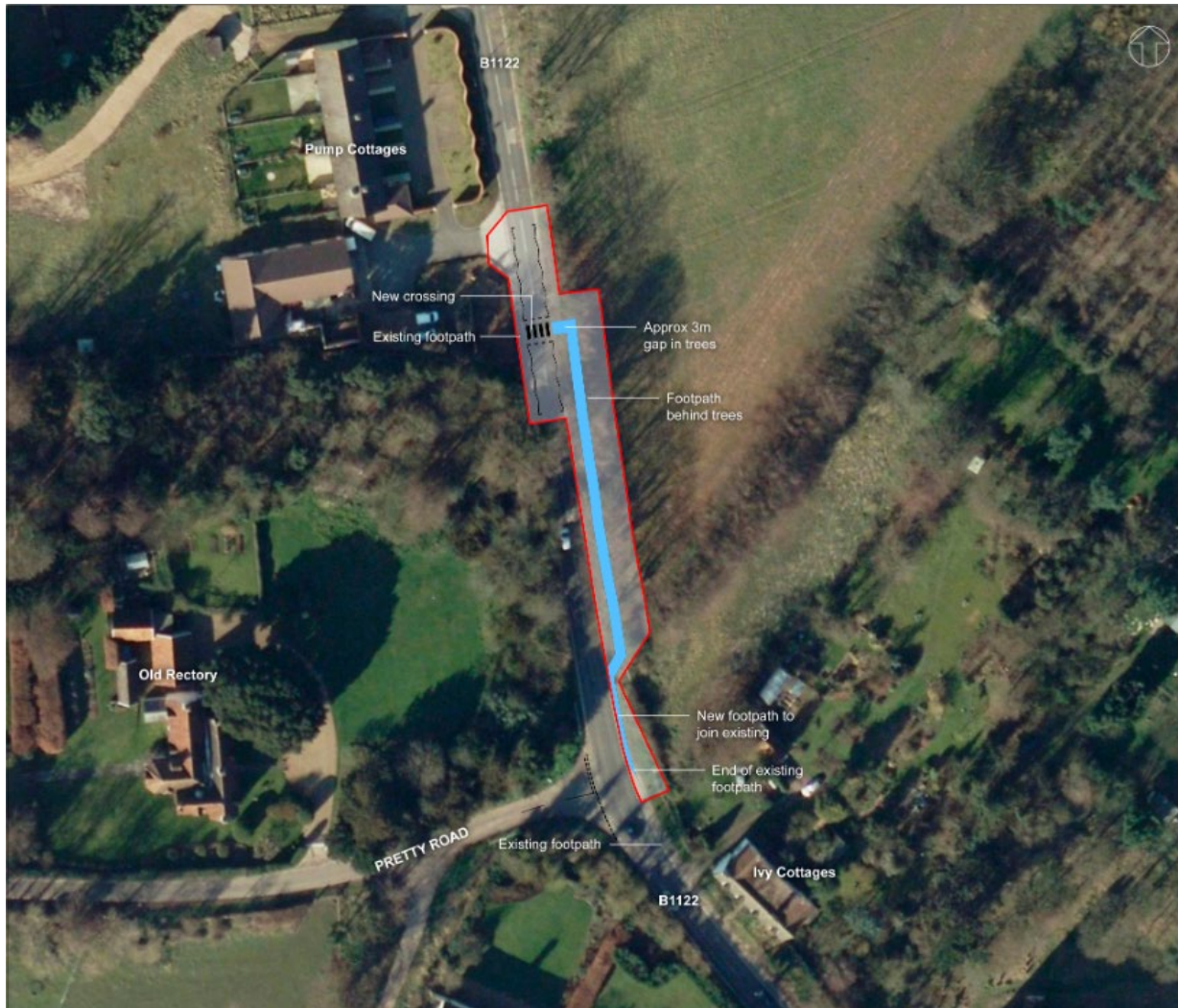
Plate 3.2 Stage 2 - Proposed pedestrian crossing and footpath at Pump Cottages, Theberton
