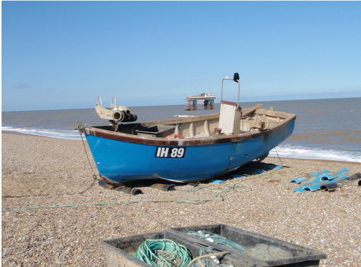
Figure 8 A commercial longshore fishing boat on Sizewell beach, equipped with gillnets and net/pot hauler
