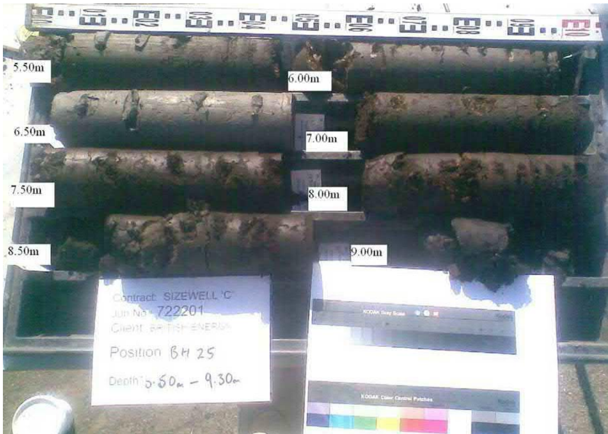
BH25 depth: 5.50m to 9.00m
