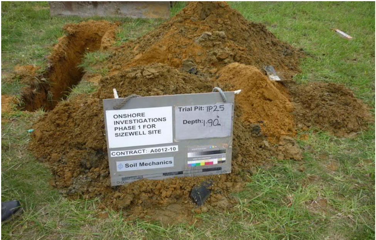
Trial Pit 25 Spoil
