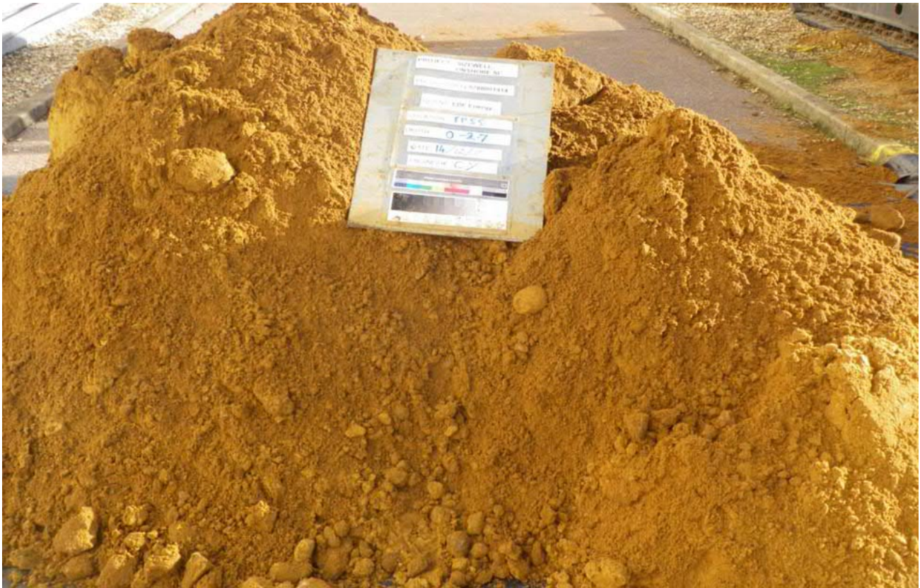
Trial Pit 55 Spoil
