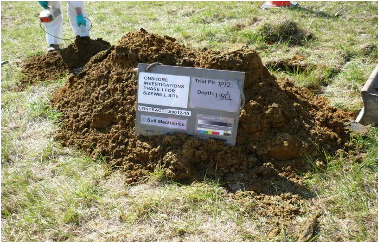
Trial Pit 12 Spoil
