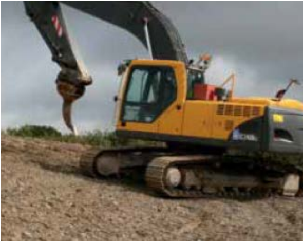
Plate 4 – Single rigid tine working
