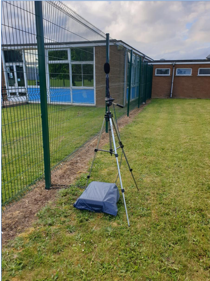
A5: Unattended survey sound level meter setup with environmental kit.
