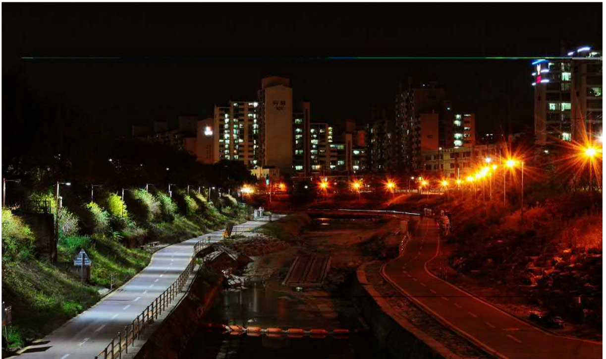
Figure 5.1: LED (left hand side) and Sodium (right hand side) Light Sources for Comparison
