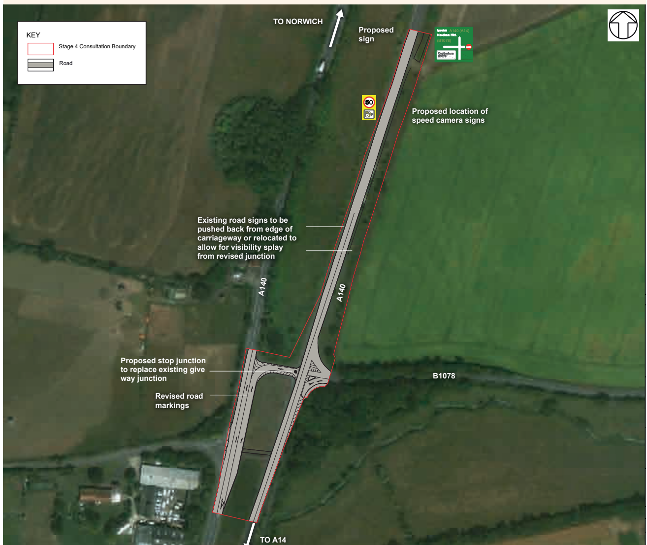
Figure 2.30: A140/B1078 west of Coddendam – proposed highway improvements
