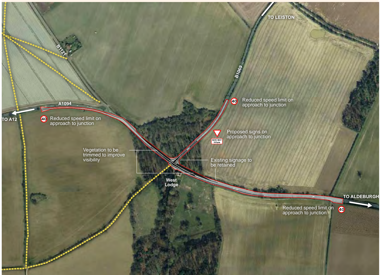
Figure 17.8 A1094/B1069 south of Knodishall – proposed highway improvements
