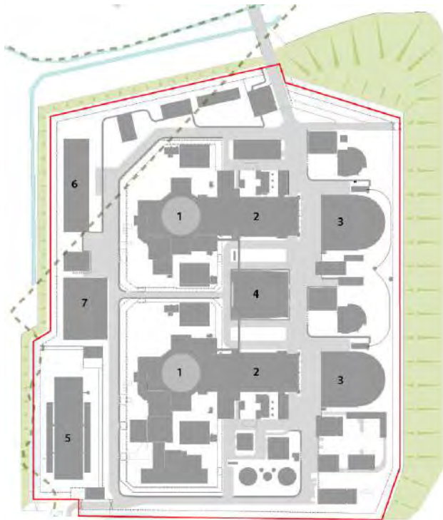
Figure 7.6 Stage 2 power station layout
