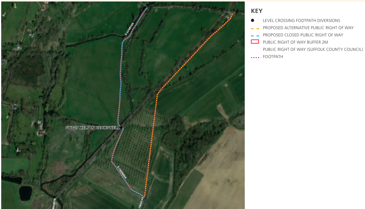
Figure 9.22 Melton Bromswell level crossing diversion Option 4
