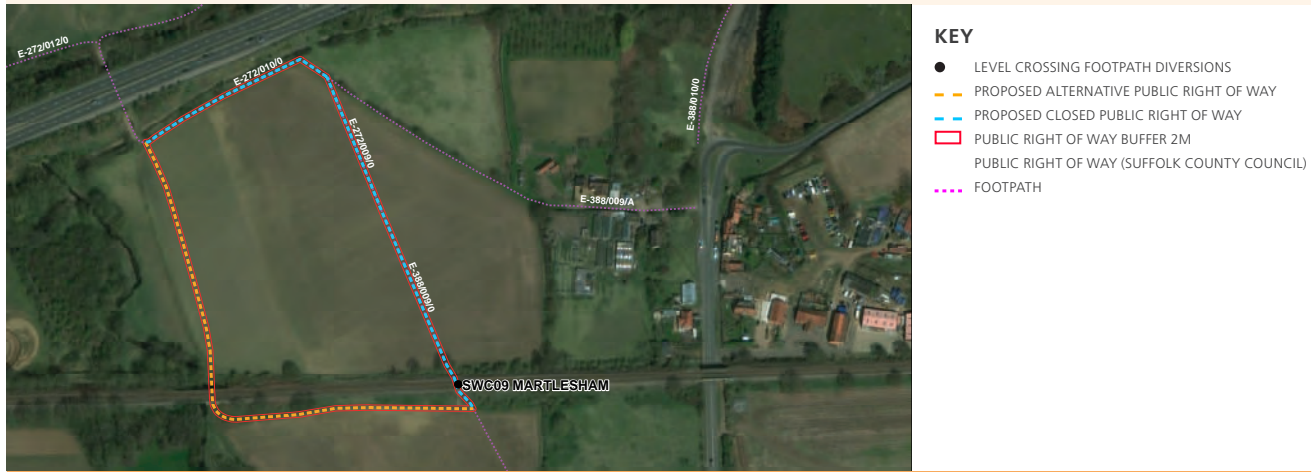
Figure 9.17 Martlesham level crossing diversion Option 2
