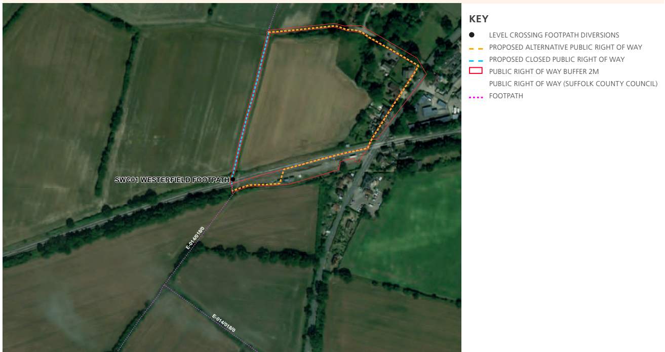
Figure 9.4 Westerfield footpath level crossing diversion Option 3
