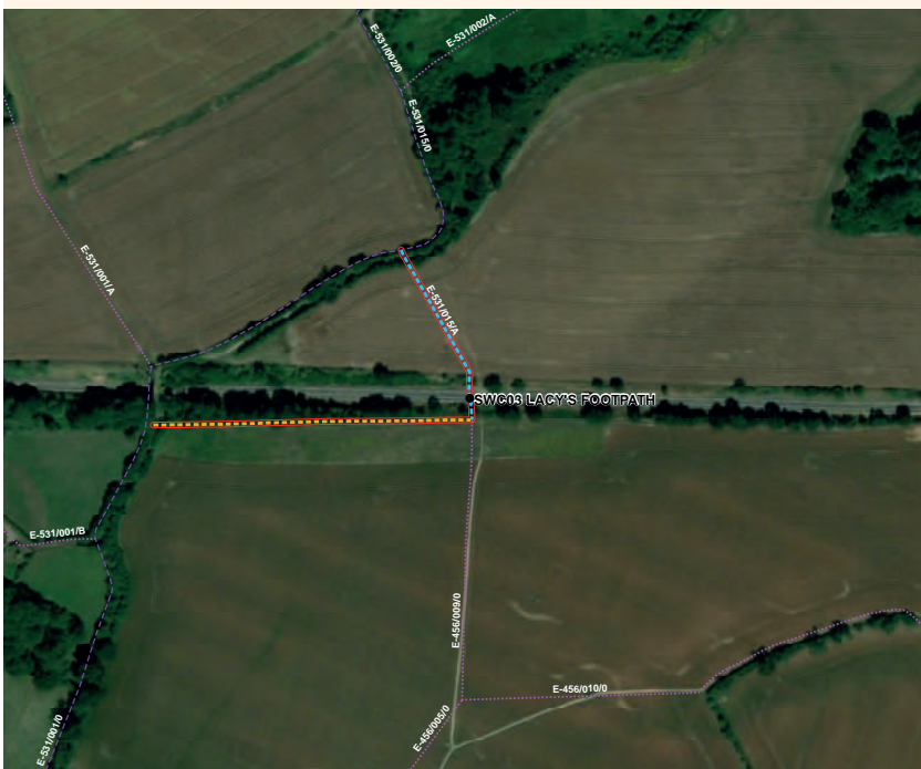
Figure 9.6 Lacy's footpath level crossing diversion route
