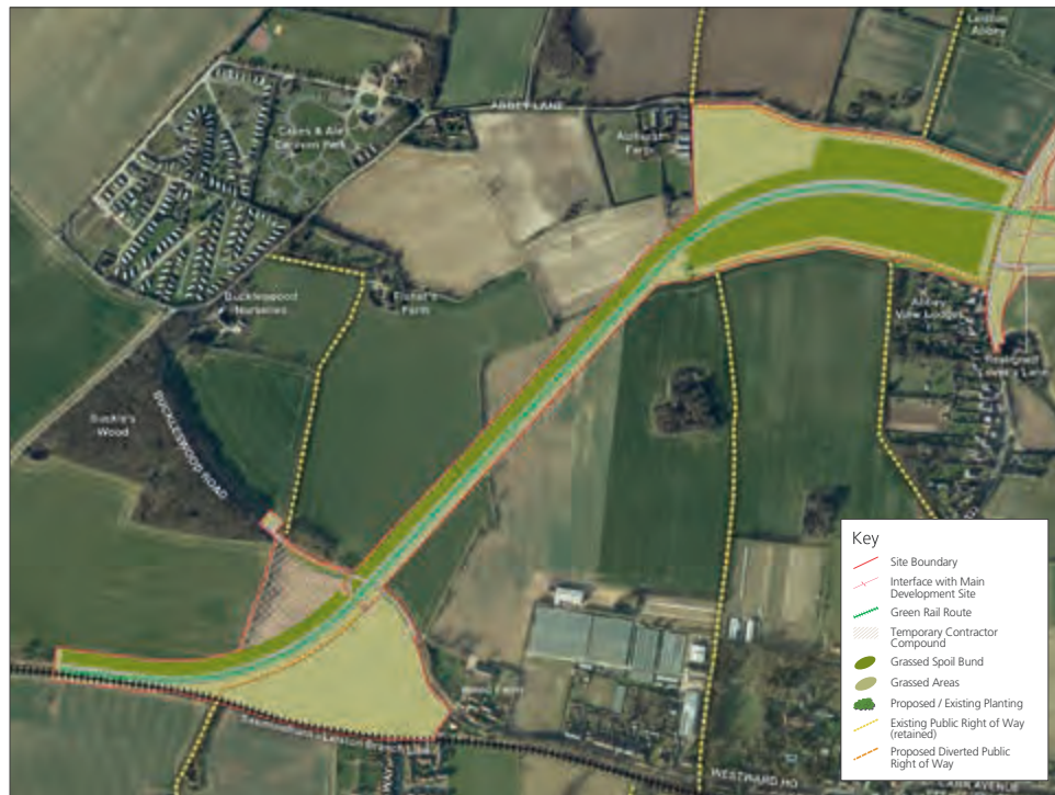
Fig 5.4: Option 1 - Illustrative route of temporary extension to Saxmundham-Leiston branch line (green route)
