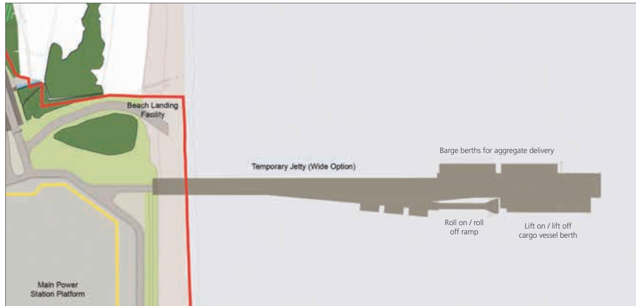
Fig 5.6: Option 1 - wide jetty (temporary)
