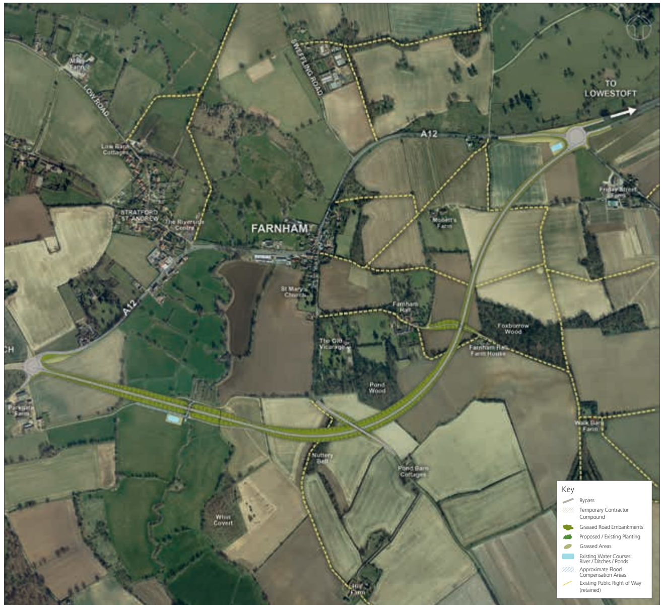
Fig 5.14: Option 4: Farnham and Stratford St Andrew bypass (a two-village bypass) (illustrative plan)
