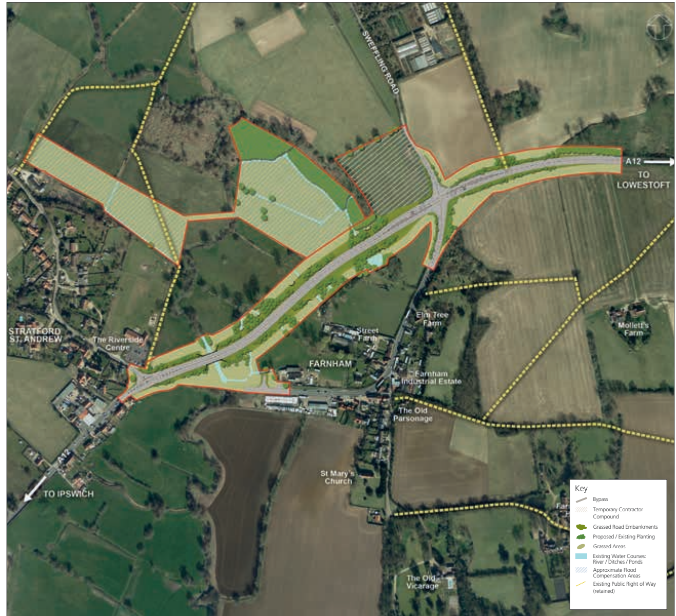
Fig 5.12: Option 3A - Joining the A12 at Sweffling Road at a signalised junction (illustrative plan)
