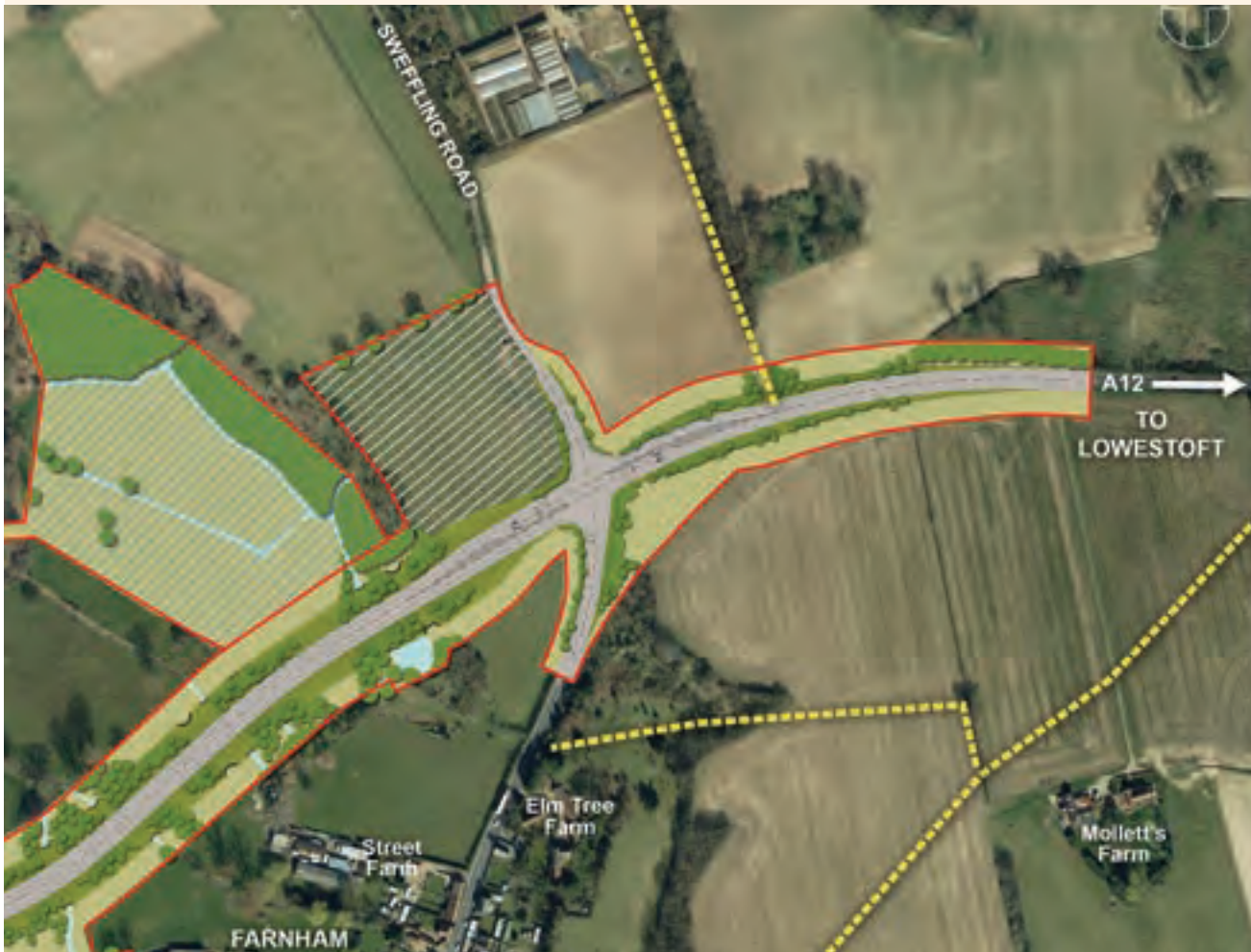
Figure 11.12 Indicative design of Option 3A: junction with the existing A12 north of Farnham
