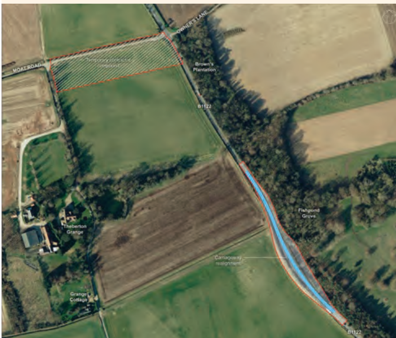
Figure 11.26 Improvement to the alignment of the B1122 between Theberton and the Sizewell C construction site entrance
