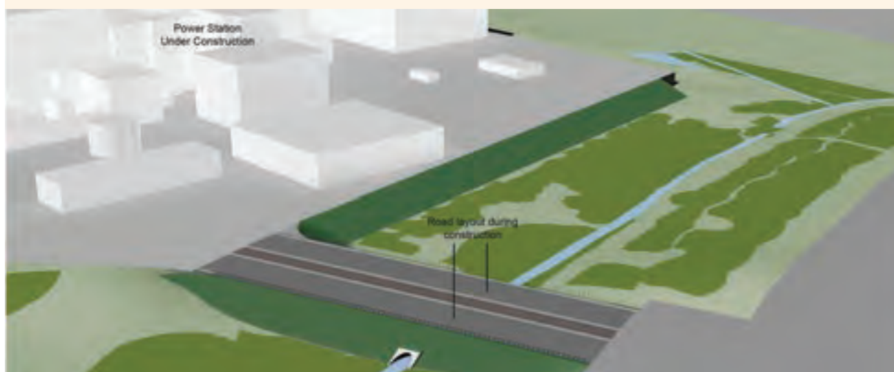
Figure 7.21 Option 1: Causeway over culvert
