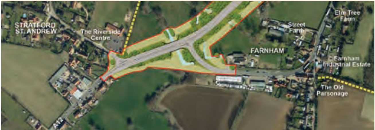
Figure 11.13 Indicative design of Option 3B: retains a connection with the existing A12
