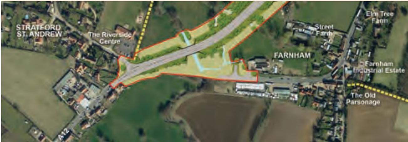
Figure 11.11 Indicative design of Option 3A: closure of the existing A12 into Farnham
