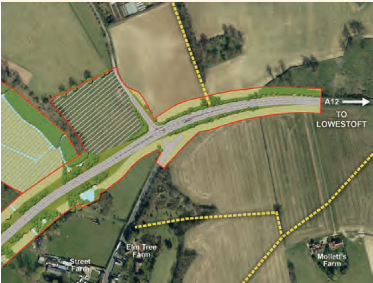
Figure 11.14 Indicative design of Option 3B: design of junction with the existing A12 north of Farnham
