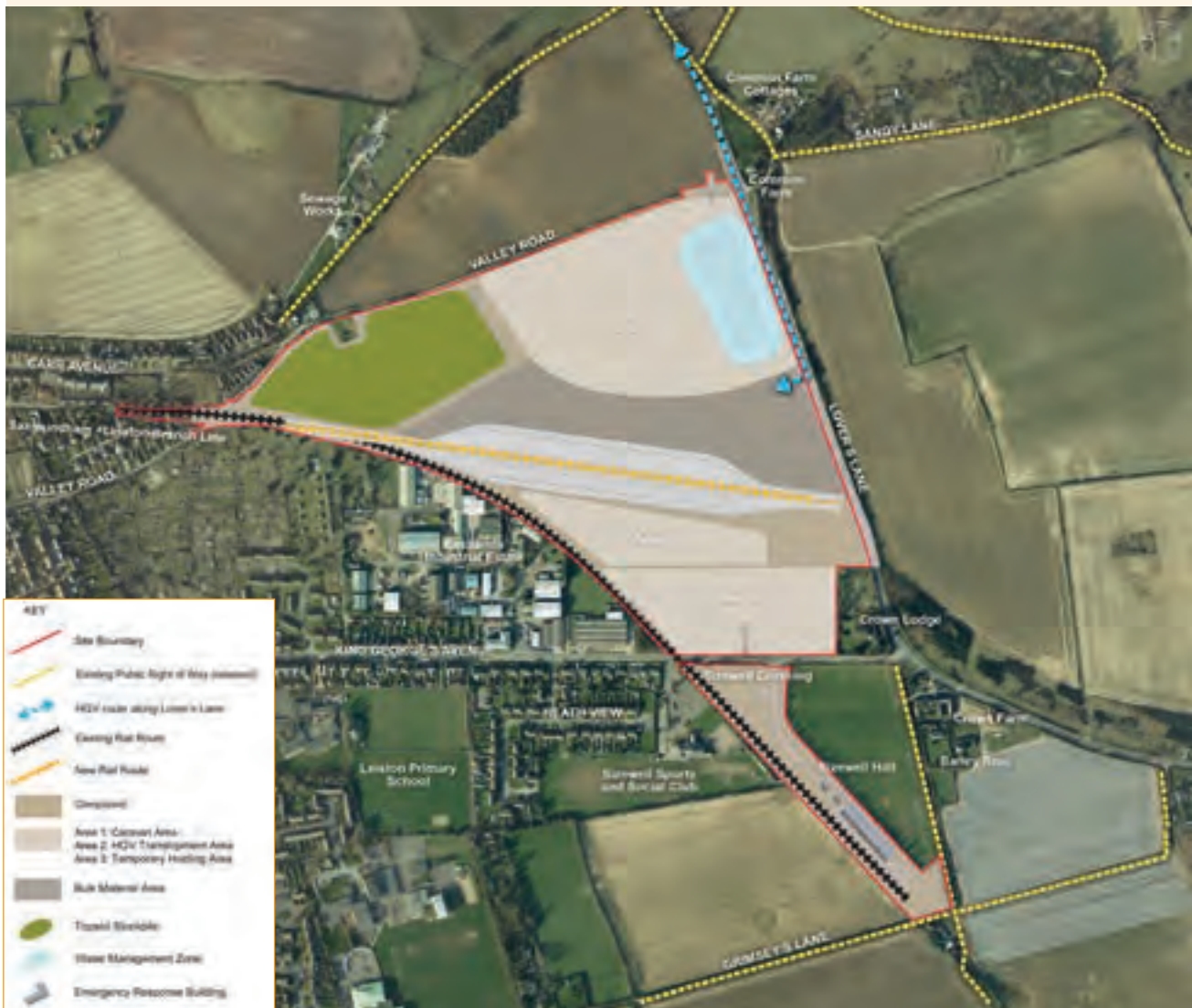
Figure 8.9 Proposed layout of the new rail terminal and freight laydown area option
